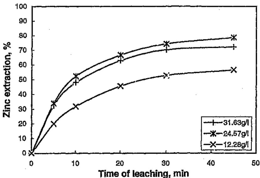
Figure 4.2 Zinc extraction into spent electrolyte containing 31.63g/l, 24.57g/l and 12.28g/l nitric acid. Conc. of  $H_2SO_4$ : 72.13g/l; Temp.: 80-90°C; pressure: 50kPa.
