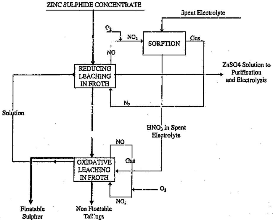
Figure 5.2 Simplified flowsheet of leaching in froth processing of zinc sulphide concentrate<sup>[39]</sup>
