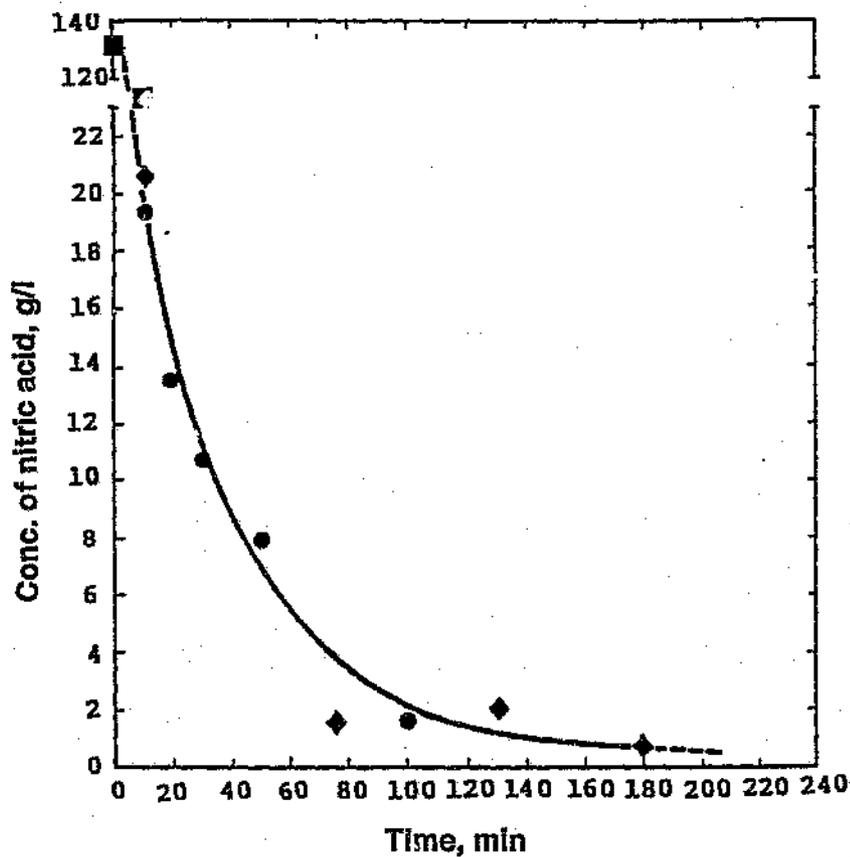
**Figure 2.3 Reduction of nitrates from leach solution by fresh concentrate in the froth<sup>[47]</sup>**
