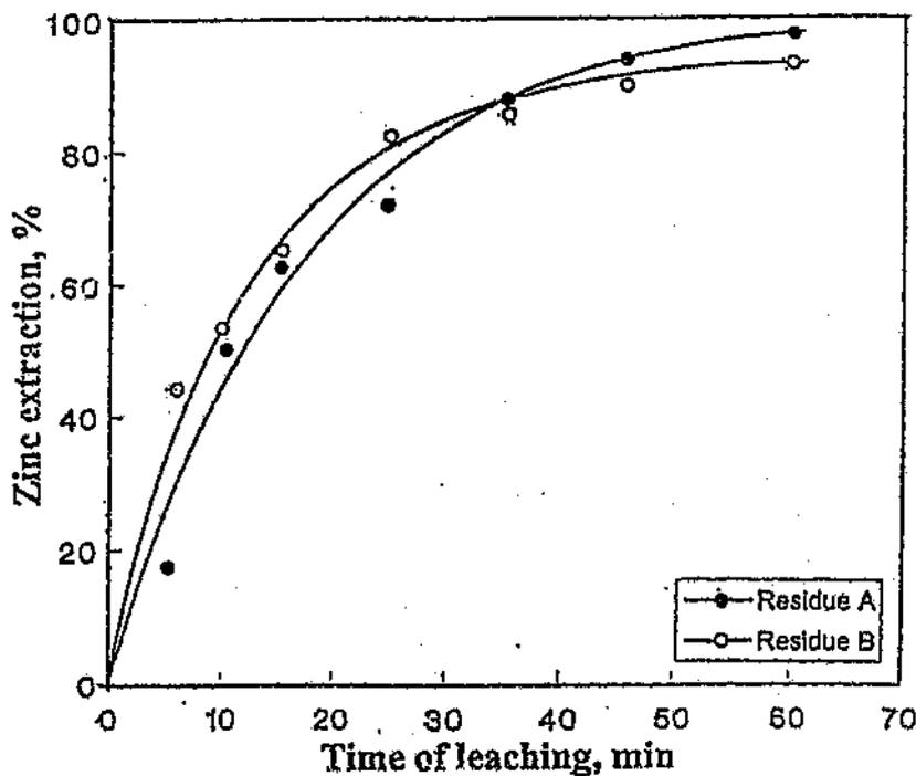
Figure 4.10 Zinc extraction during leaching of residues obtained from L/F experiments in the batch reactor. S/L ratio: 51g/l; Temp.: 80-95°C; pressure: atmospheric; stirrer speed: 400rpm.
