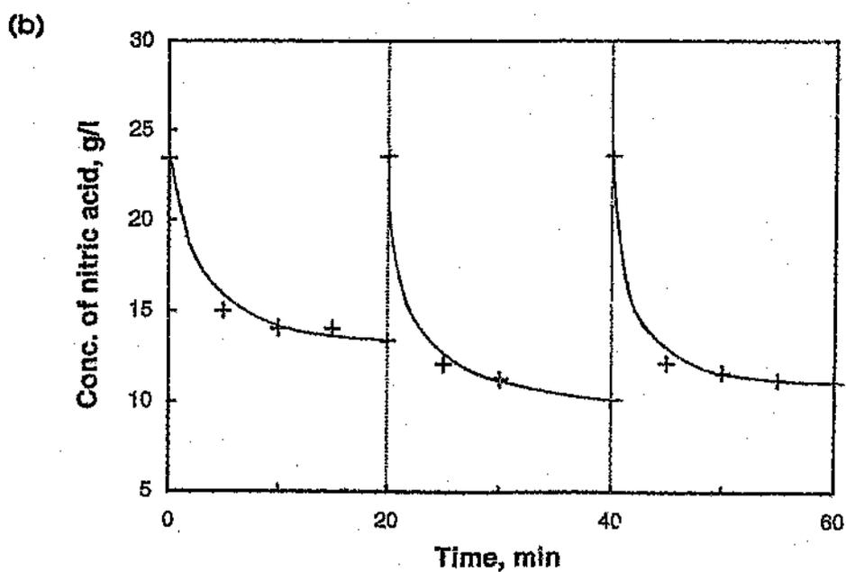
Figure 4.7 (a) Zinc extraction and (b) regeneration of nitric acid during continuous leaching in froth. Temp.: 80-90°C; pressure: 150-200kPa.
