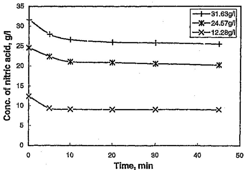
Figure 4.3 Nitric acid regeneration during zinc extraction into spent electrolyte containing 31.63g/l, 24.57g/l and 12.28g/l nitric acid. Temp.: 80-90°C; conc. of  $H_2SO_4$ : 72.13g/l; pressure: 50kPa.
