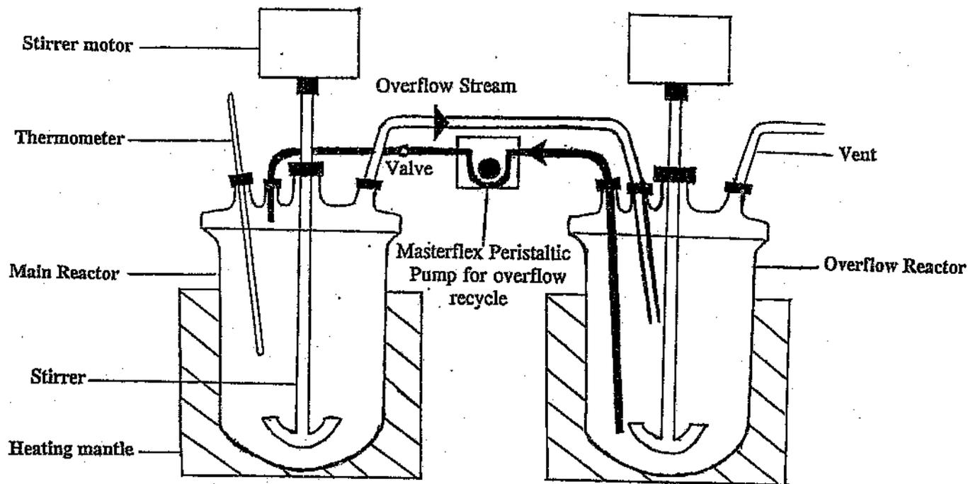
Figure 3.1 Experimental set-up of the batch reactor
