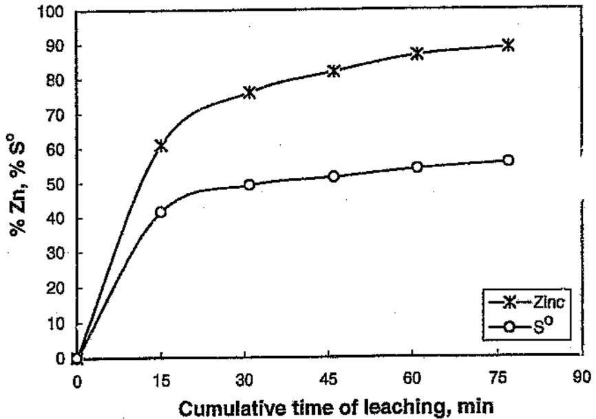
Figure 4.8 Cumulative percentage zinc extraction and elemental sulphur generated during 5-stage leaching in froth processing. Temp.: 80-90°C; pressure: 100-200kPa.
