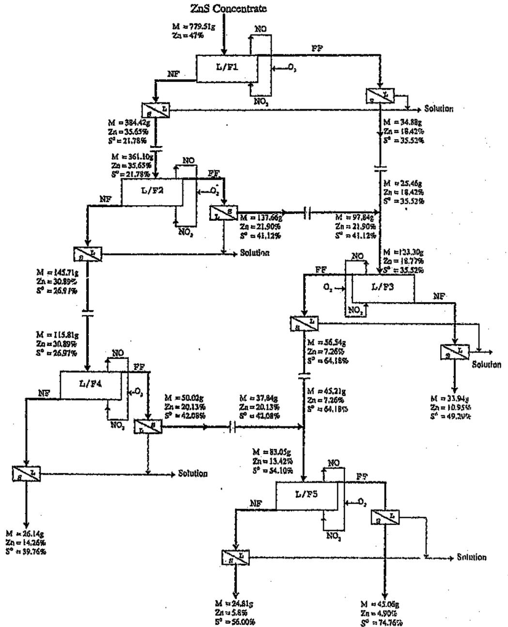
Figure 4.9 Simplified flowsheet of the 5-stage L/F processing
