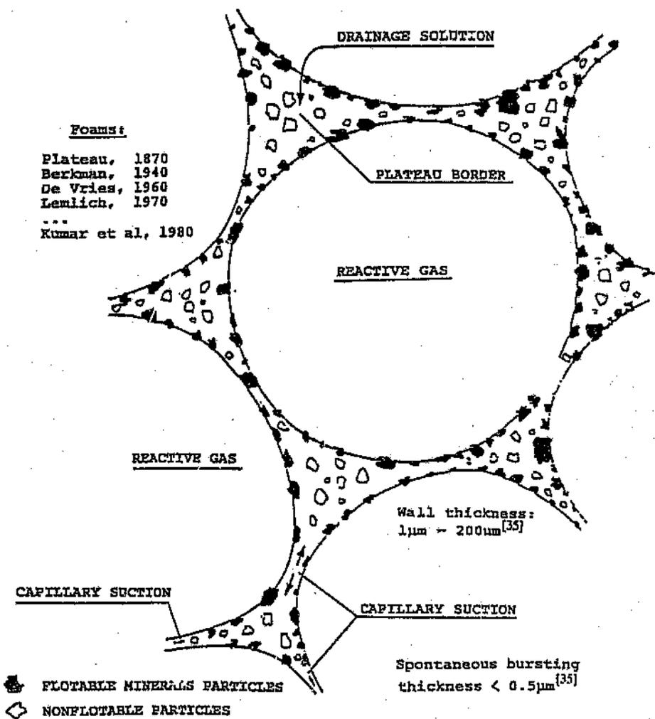
Figure 2.1 Schematic representation of a cross-section of the reactive froth fragment<sup>[28]</sup>
