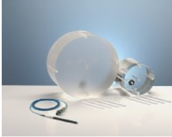
Figure 2 PTW CT ion chamber with body phantom, Ø32 cm and head phantom, Ø16 cm, both acrylic cylinders of 15 cm height. Both have holes drilled peripherally and centrally to accommodate the ionisation chamber.
