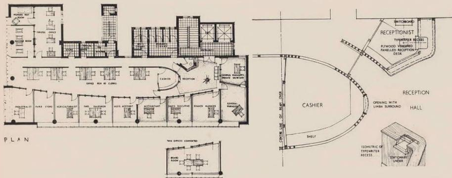
the external ply having a Kiaat veneer. Vertical cover strips of  $\frac{3}{4}$  in. by  $\frac{1}{4}$  in. Limber were used. The cashier's hatch has a Limber surround and bronze grill. A 3 in. flexible bronze skirting was used without a quadrant in order to take up the curve of the partition at floor level. A similar construction was used for the curved face of the Receptionist's desk. A wine red Axminster carpet with a heavy pile and underfelted was used in the
