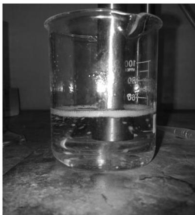
**Figure 4.5: Cavitations formed on sonication**
