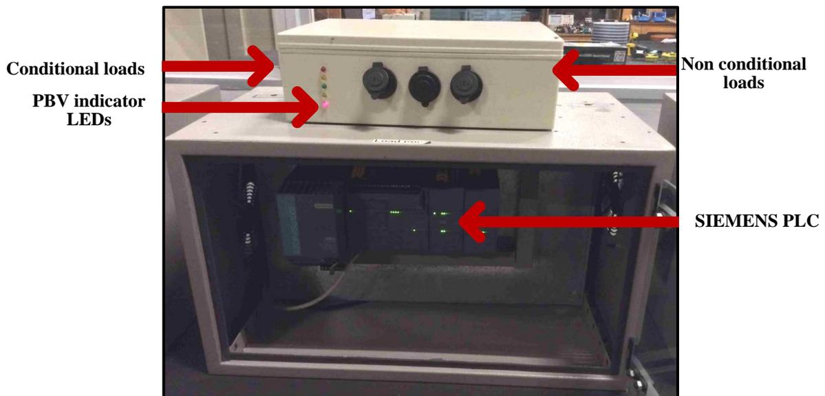
Figure 19: Load node picture
