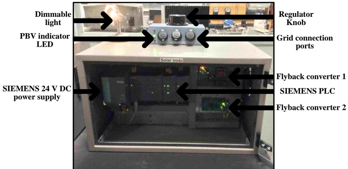
Figure 15: Solar node photograph
