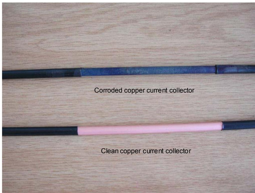
Figure A2 Corroded copper current collector shown after Run 1
