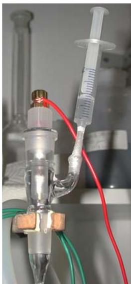
**Figure 4.3** Modified salt bridge containing reference electrode
