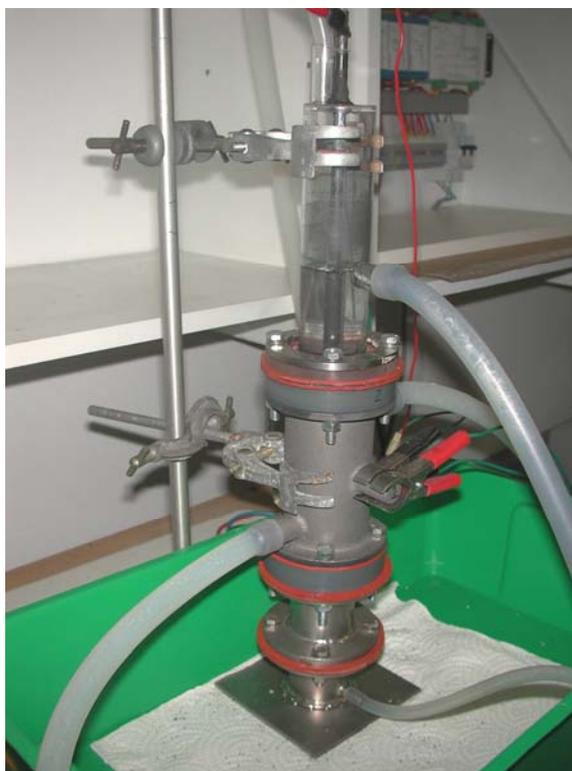
Figure A1 Photograph of the benchscale electrochemical reactor
