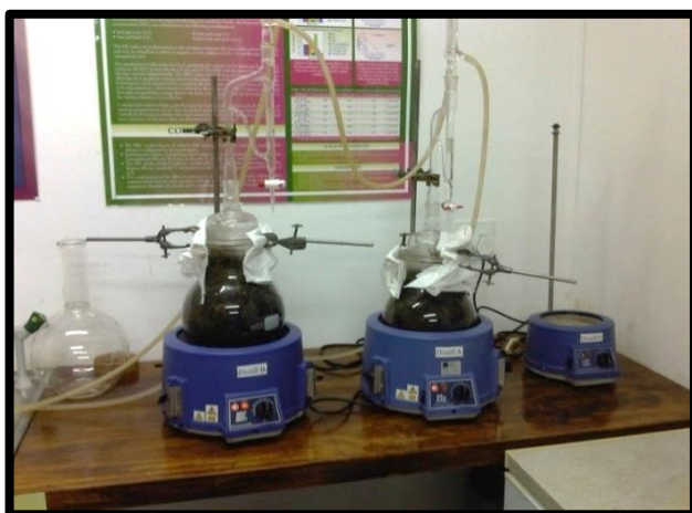
Figure 2.1. Essential oil distillation for A. afra , using a Clevenger-type apparatus.
