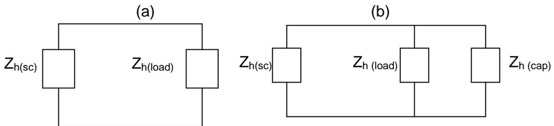
Figure 4.7: (a) Equivalent network diagram without any shunt compensation
