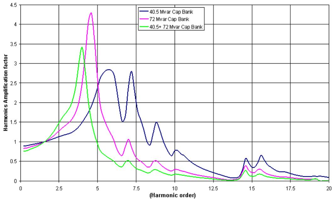
Figure 3.16: Komatipoort 132kV busbar harmonic impedance plots for various shunt capacitor bank sizes.
