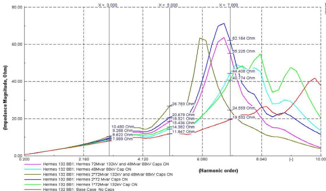
Figure 5.21: Hermes 132kV busbar harmonic impedance plots
