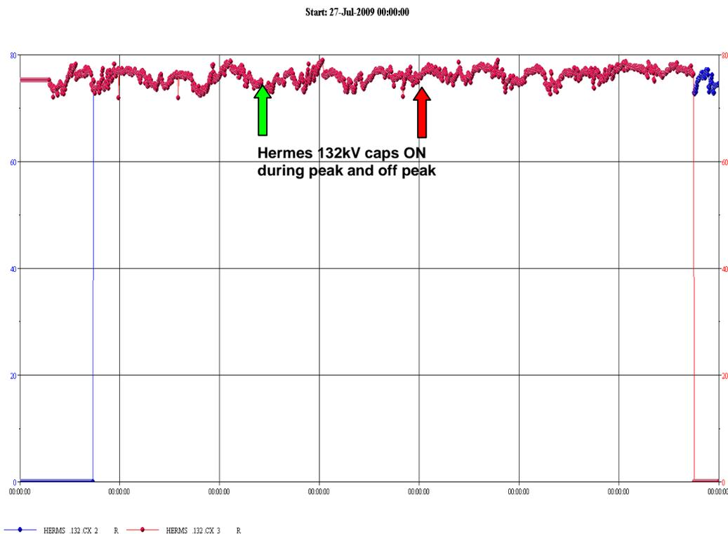
Figure 5.19: Hermes 2x72 MVar capacitor bank MVar profiles.
