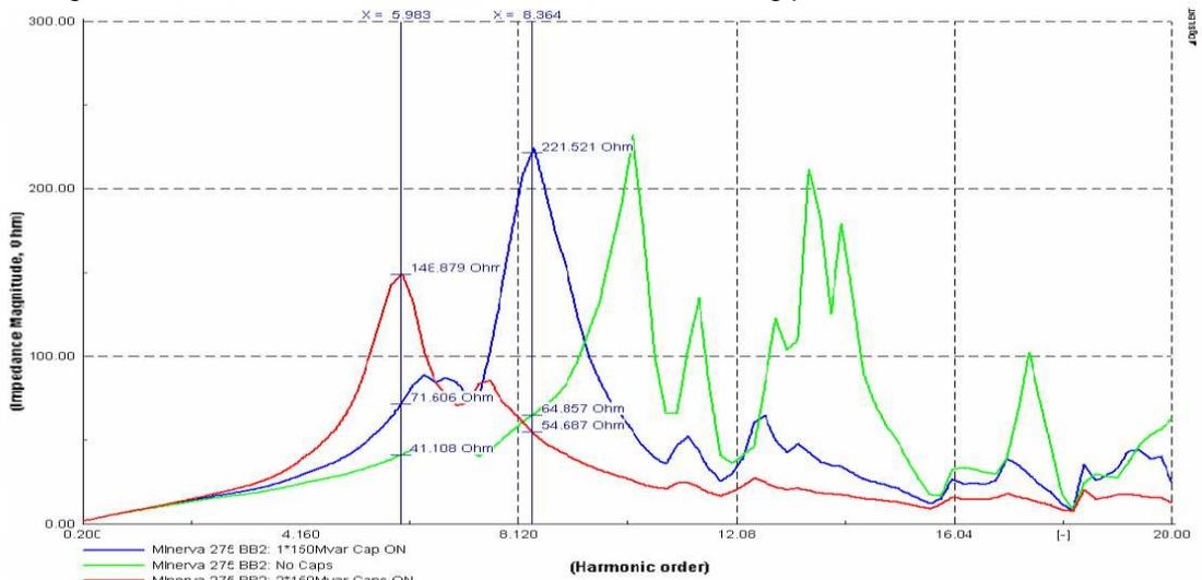
Figure 5.10: Minerva 275kV busbar harmonic impedance plots
