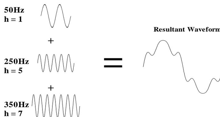
Figure 2.1: Distorted sinusoid
