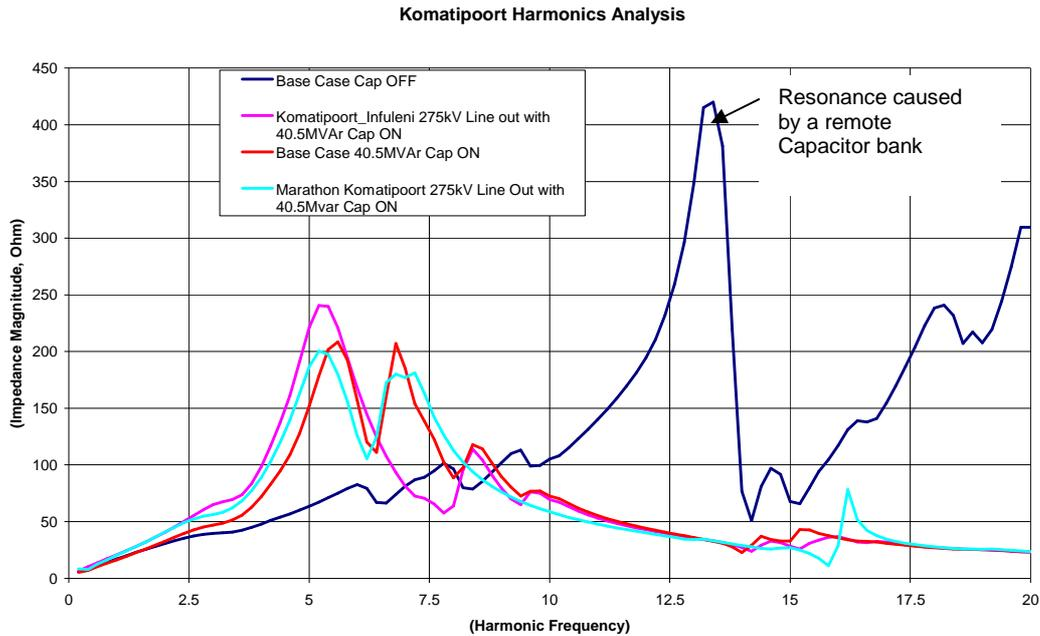
Figure 3.17: Komatipoort 132kV busbar harmonic impedance plots for various network contingencies
