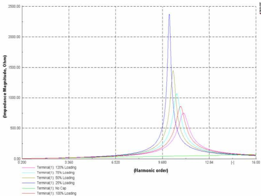
Figure 3.14: Makalu 275kV busbar harmonic impedance plots for different loading patterns
