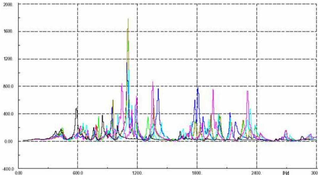
Figure 4.1: Impedance plots for various system contingencies: 150 MVA capacitor bank [2]
