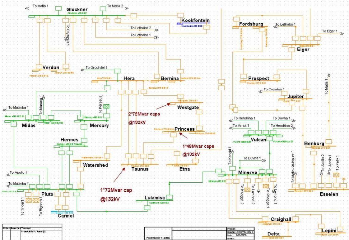
Figure 5.11: Simplified Westgate network diagram
