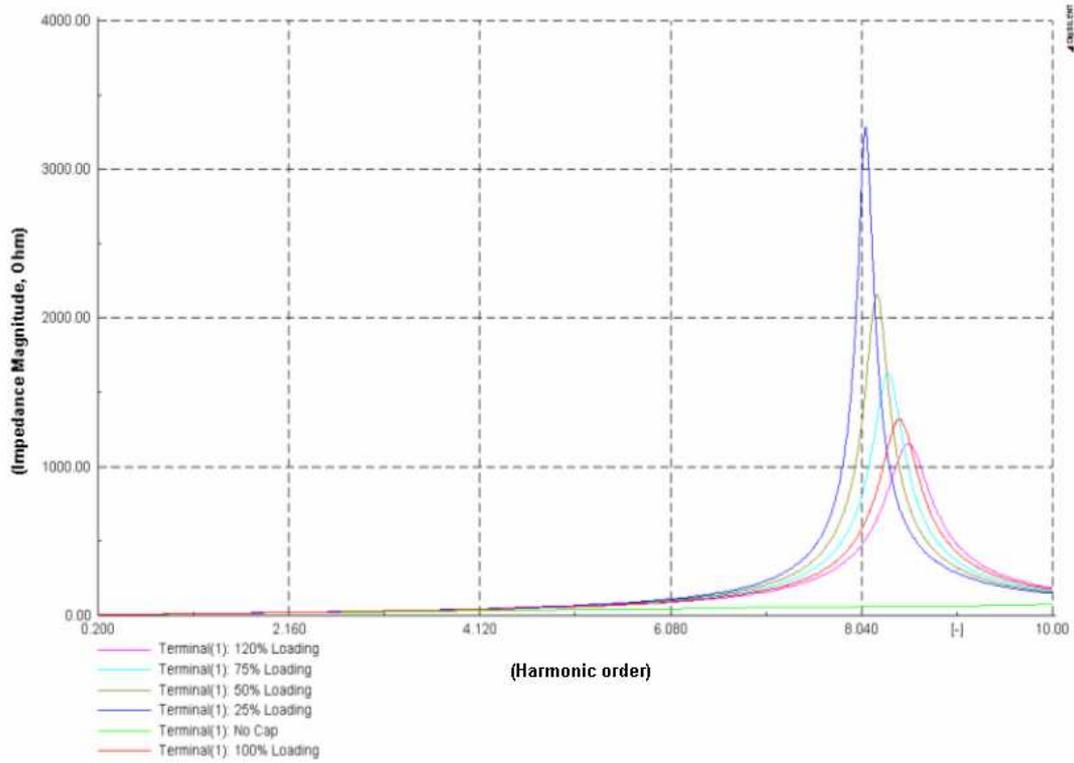
Figure 3.13: Komati 275kV busbar harmonic impedance plots for different loading patterns
