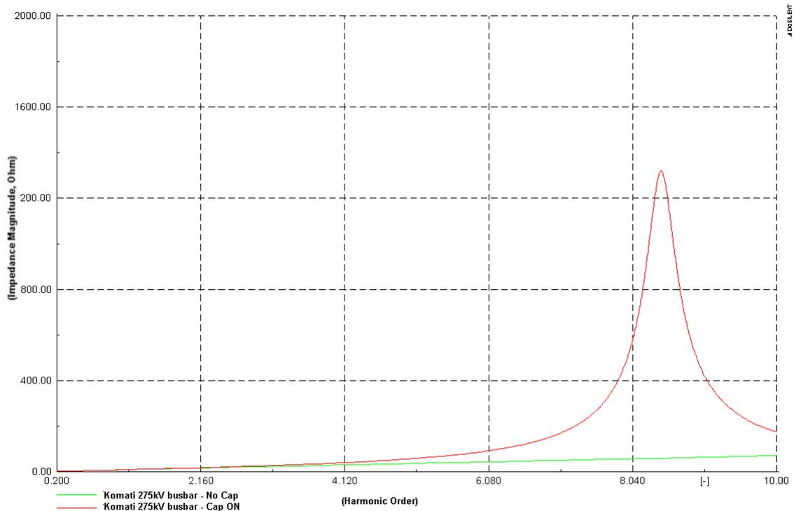
Figure 3.10: Komati 275kV busbar harmonic impedance plots
