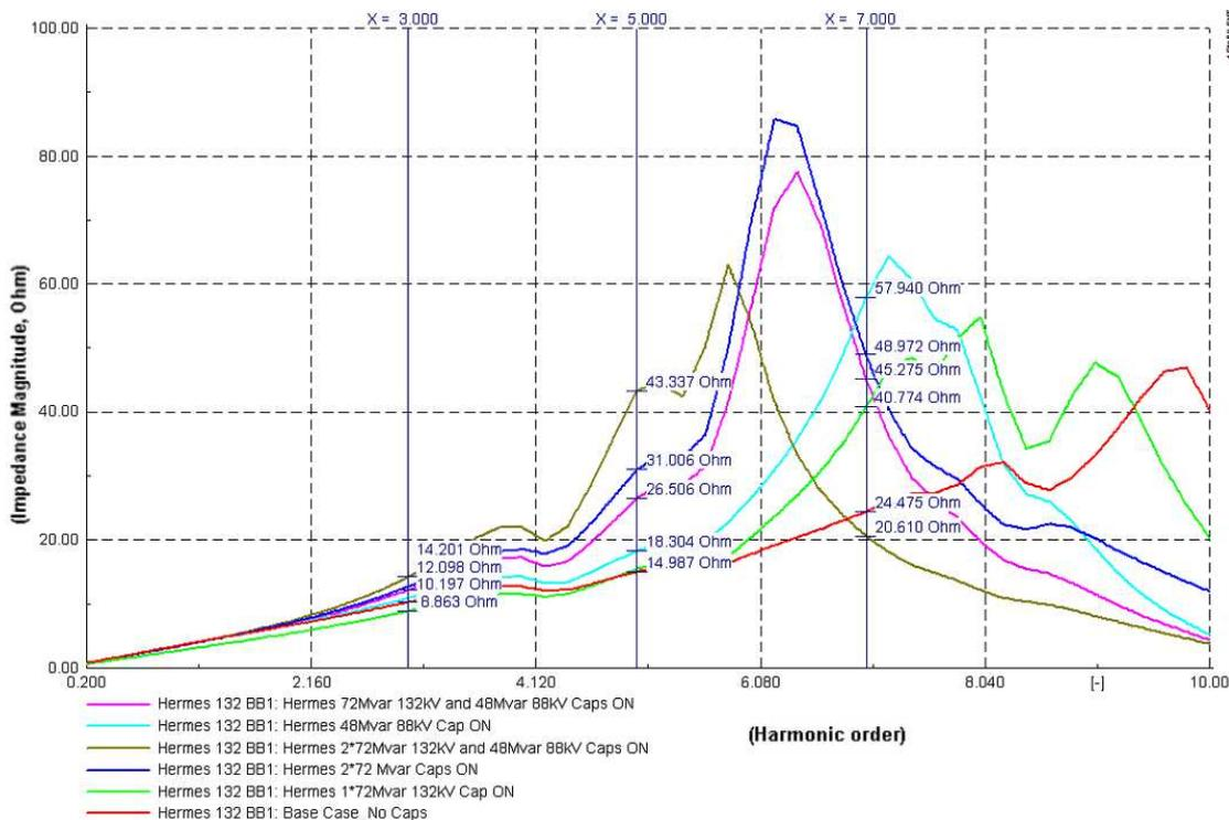
Figure 5.22: Hermes 132kV busbar harmonic impedance plots with transformer 2 out of service
