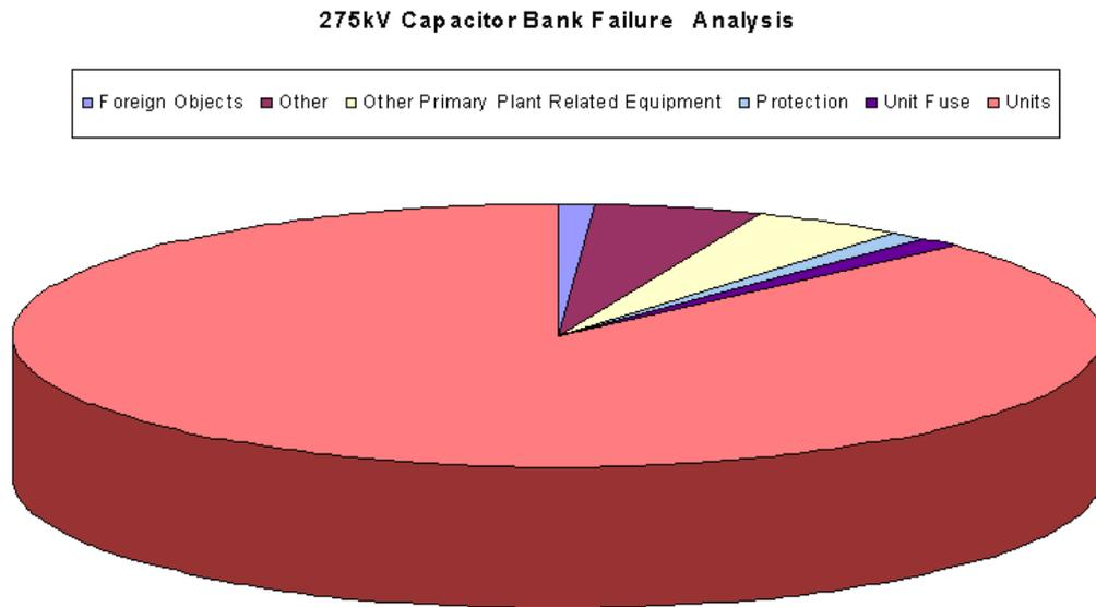
Figure 7.8: 275kV plain capacitor banks - root cause analysis
