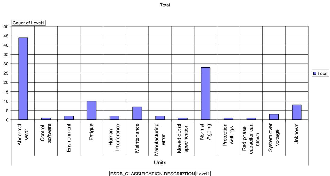
Figure 7.9: Breakdown of unit failures for EHV shunt capacitor banks
