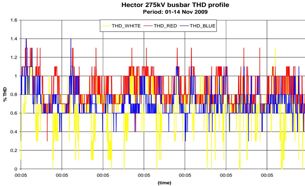
Figure 5.2: Hector 275kV busbar voltage harmonic profile
