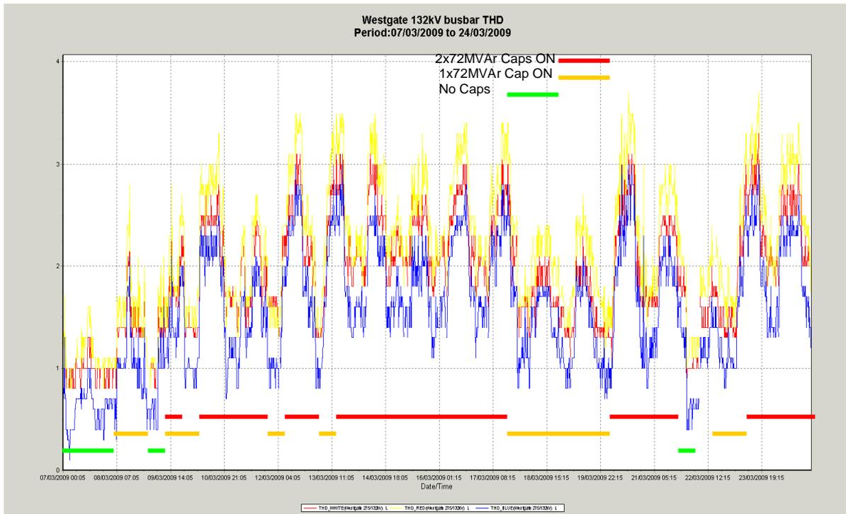
Figure 5.12: Westgate 132kV bus THD measurements and capacitor bank switching
