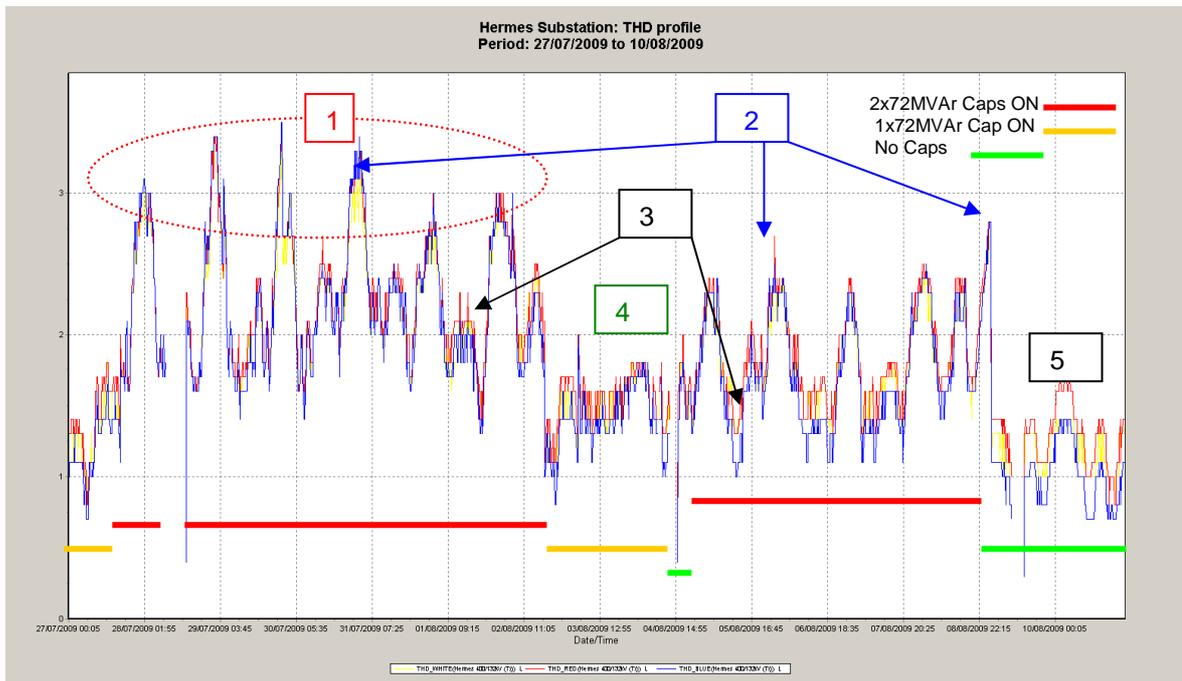
Figure 5.18: Hermes 132kV bus THD measurements and capacitor banks switching
