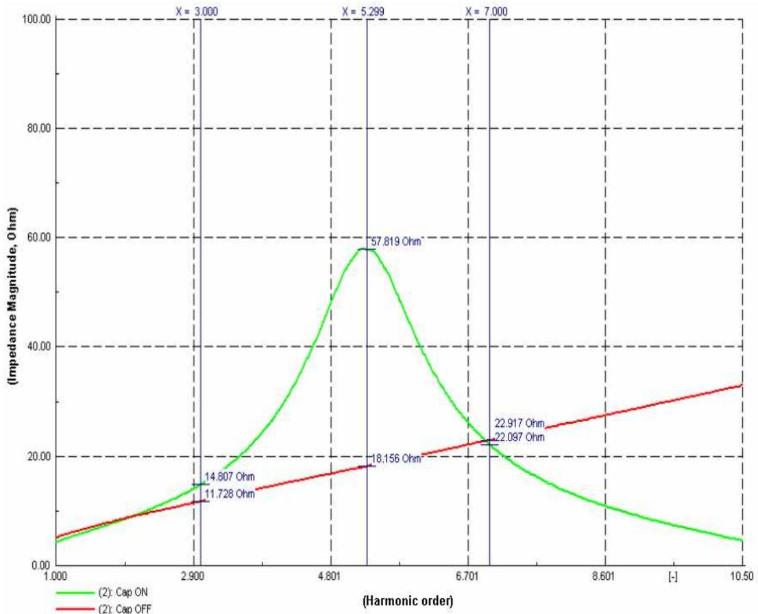
Figure 3.5: Harmonic impedance plots illustrating harmonic amplification and resonance when a capacitor bank is switched on.
