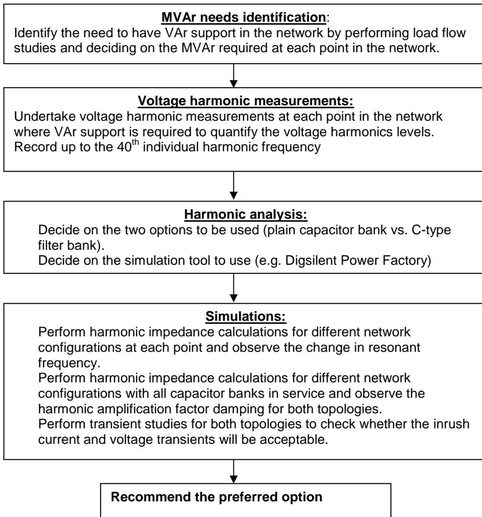
Figure 4.3: Flow-chart from the guidelines for the implementation of VAr support in the Dutch Transmission network, derived from [2]
