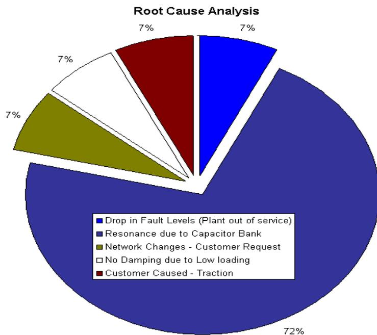
Figure 1.3: Root cause analysis for high THD levels in Eskom Transmission networks for 2008-2009 financial year [17]
