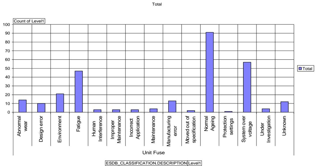
Figure 7.3: Breakdown of unit fuse failures in HV shunt capacitor banks
