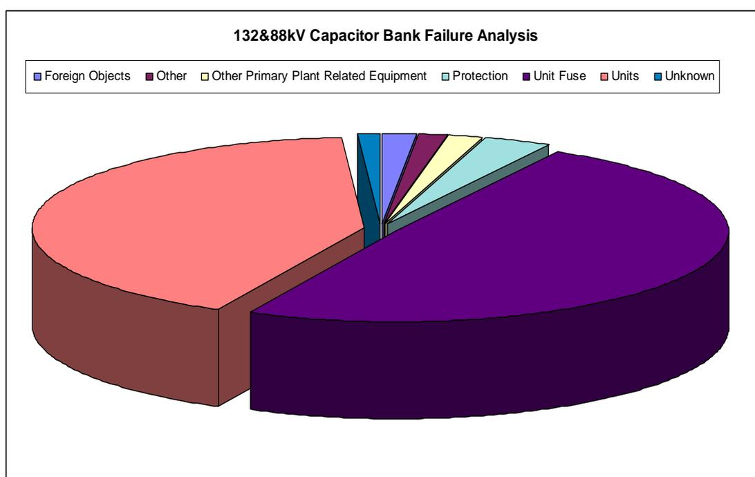
*Figure 7.2: 132kV and 88kV plain capacitor banks - root cause analysis*
