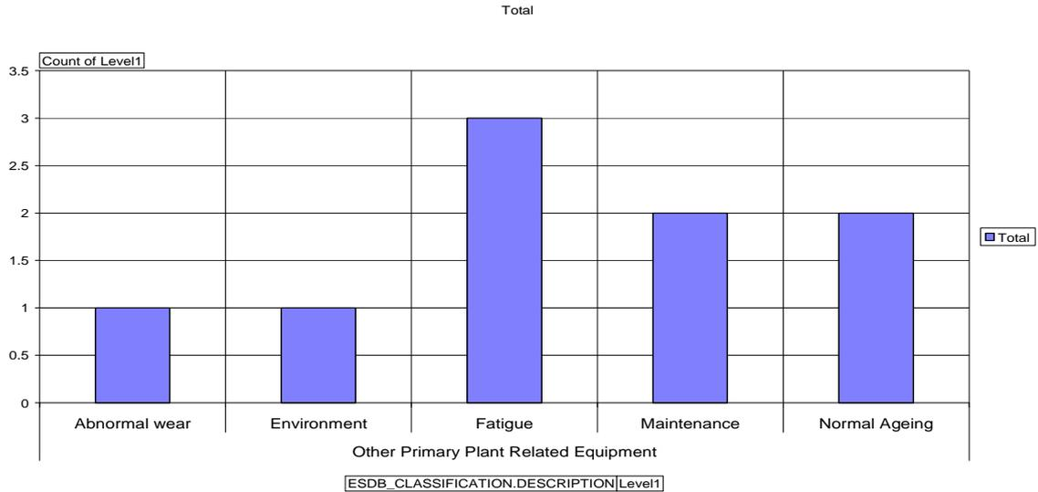
Figure 7.6: Breakdown of other primary plant related equipment for HV shunt capacitor banks.
