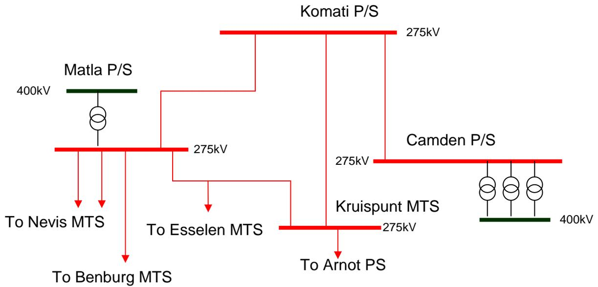
Figure 3.7: Simplified Komati network diagram
