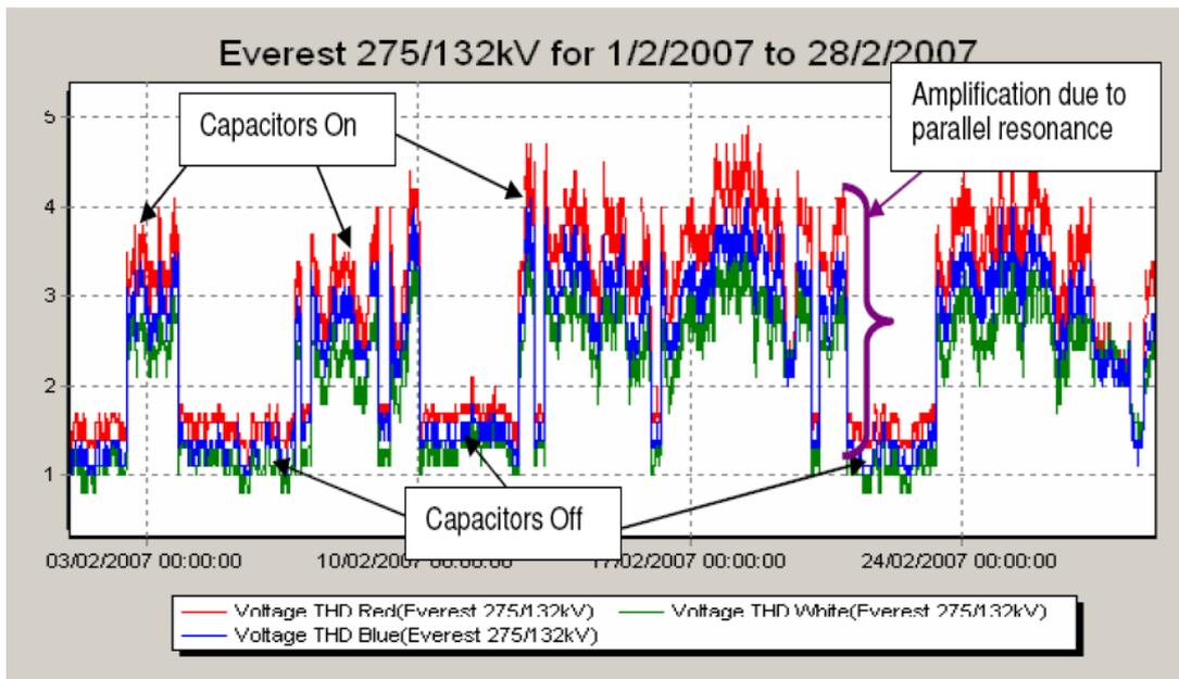
Figure 1.1: High levels of THD due to a parallel harmonic resonance caused by the switching of a capacitor bank at Everest substation
