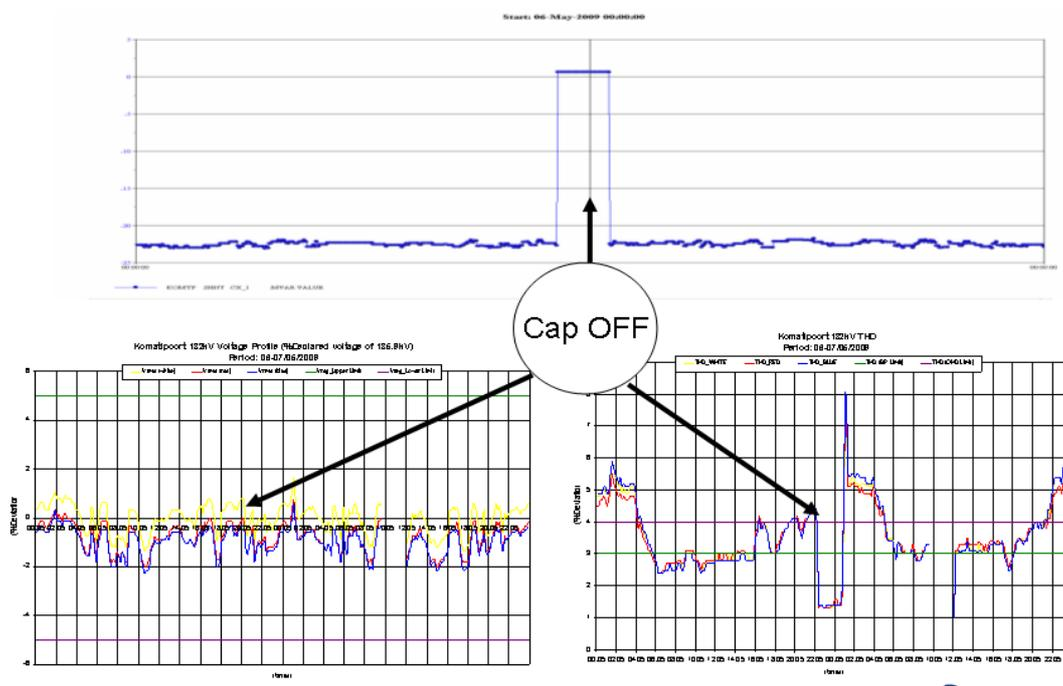
Figure 3.20: Komatipoort 132kV busbar measurements illustrating cap off at night.
