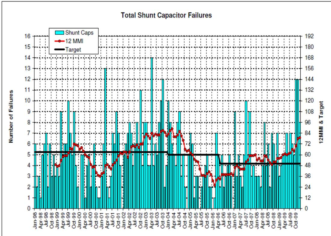
Figure 7.1: Total shunt capacitor banks failures [26]
