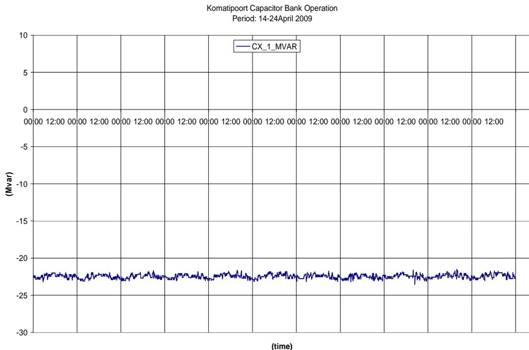
Figure 3.22: Komatipoort 132kV capacitor bank MVar measurements.
