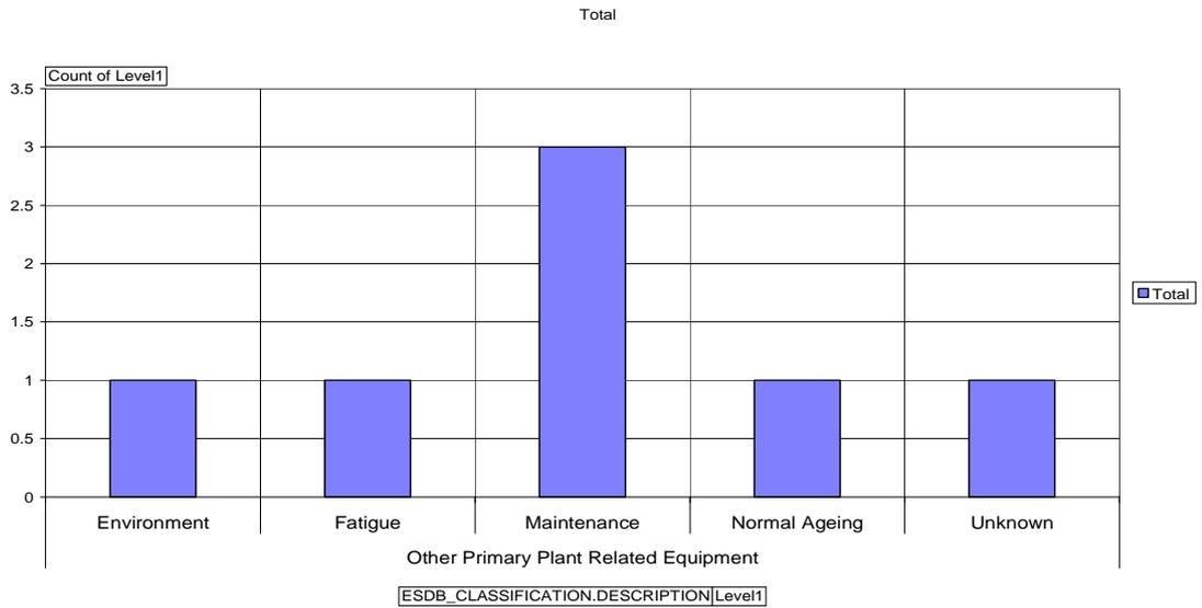
Figure 7.10: Breakdown of other primary plant related failures on EHV shunt capacitor banks
