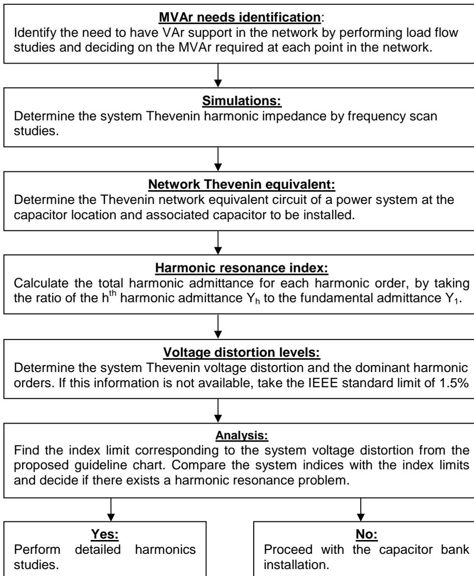
Figure 4.6: Flow-chart for the assessment of harmonic resonance problems, derived from [5]
