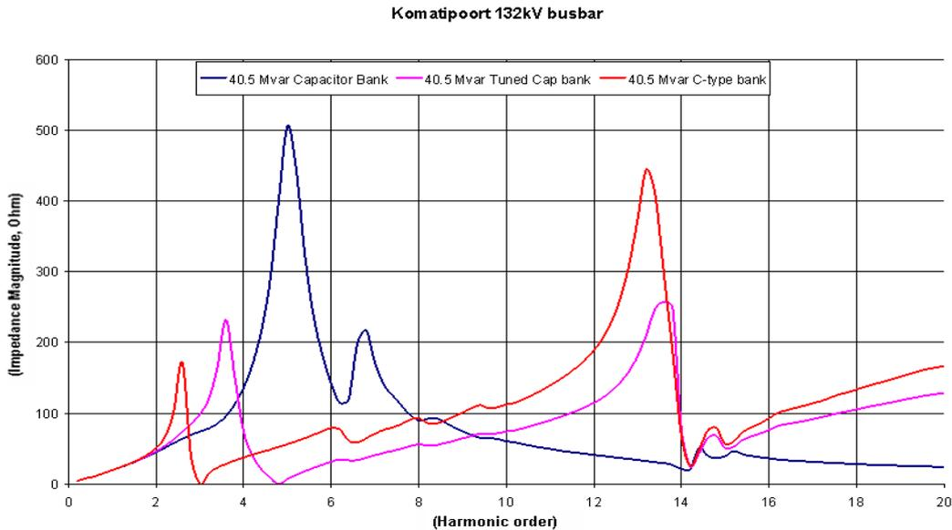
Figure 3.18: Komatipoort 132kV busbar harmonic impedance plots for different shunt capacitor bank technologies.
