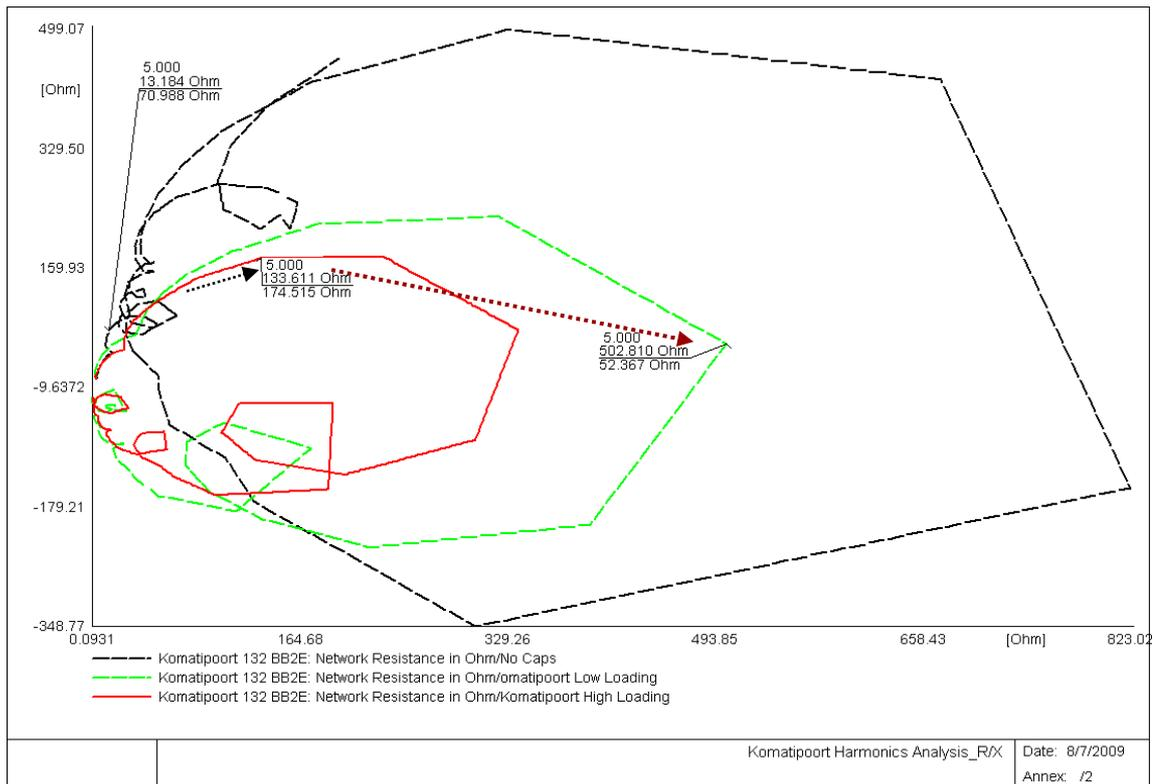
Figure 3.24: Komatipoort 132kV busbar R/X polar plots with the 40.5 MVar shunt capacitor bank switched for various loading patterns.
