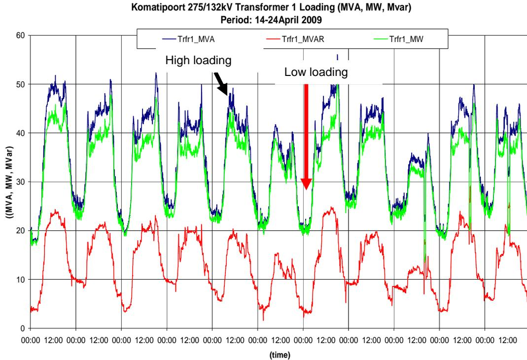
Figure 3.21: Komatipoort transformer 1 loading (apparent, active and reactive power) measurements.
