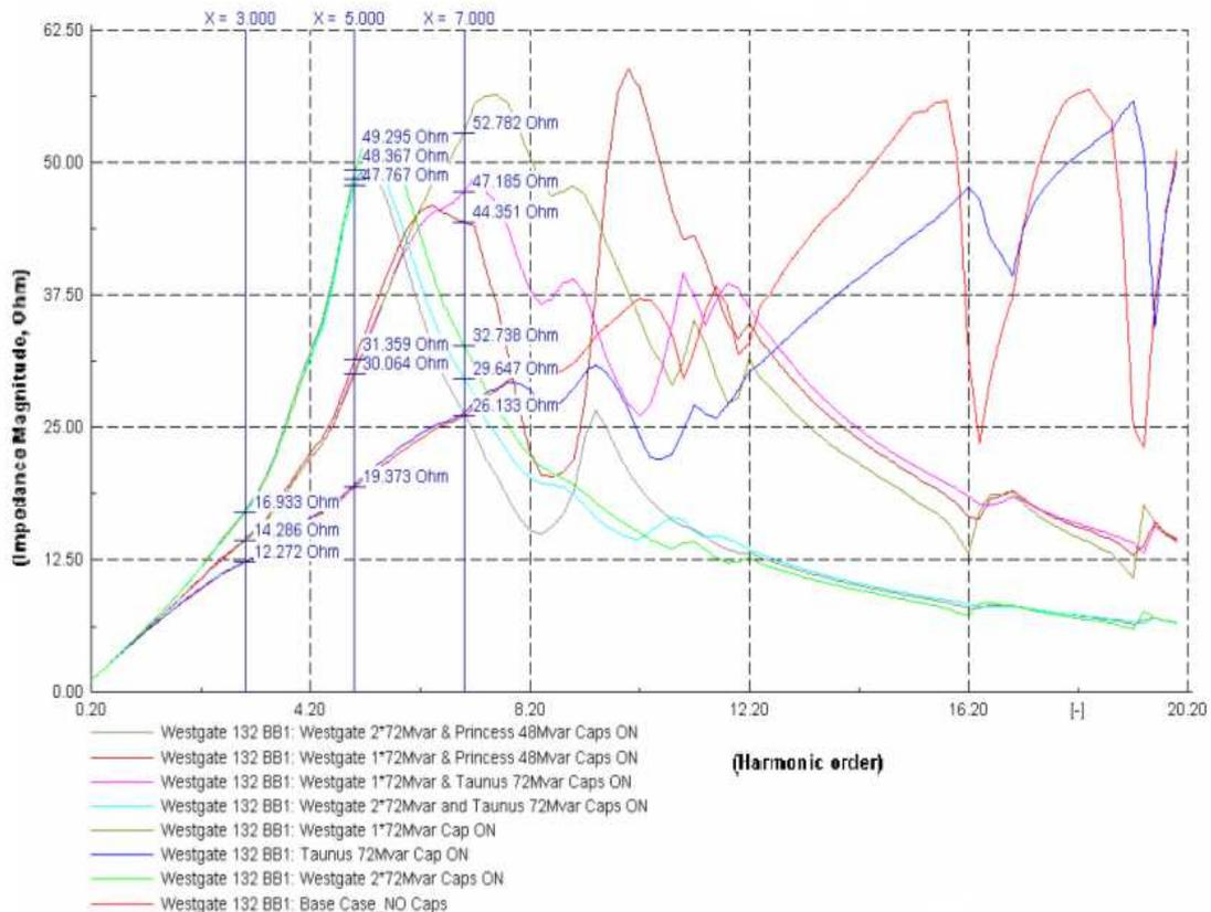
Figure 5.15: Westgate 132kV busbar harmonic impedance plots
