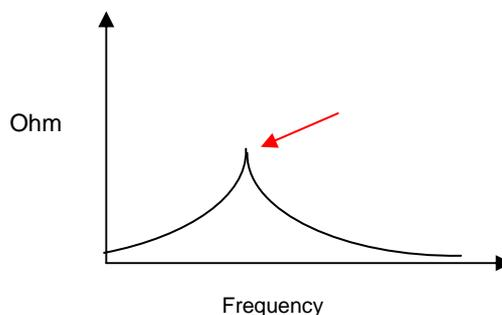
Fig. 3.4: Parallel resonance
