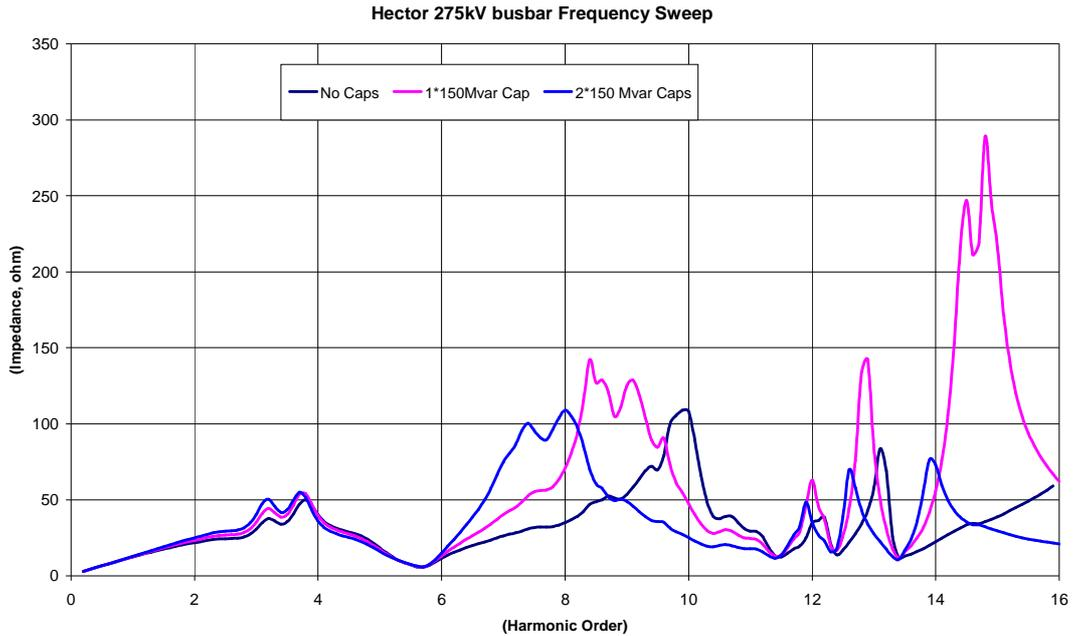
Figure 5.5: Hector 275kV busbar harmonic impedance plots.
