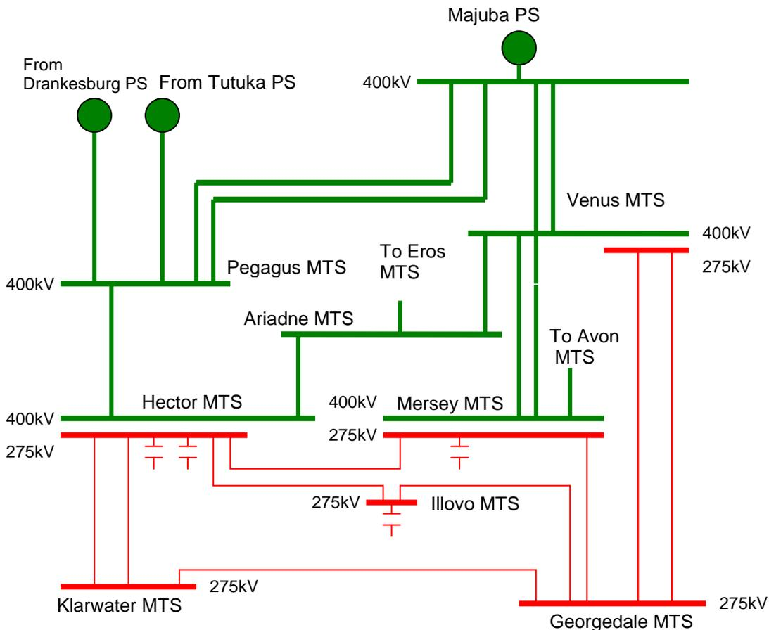
Figure 5.1: Simplified Hector network diagram
