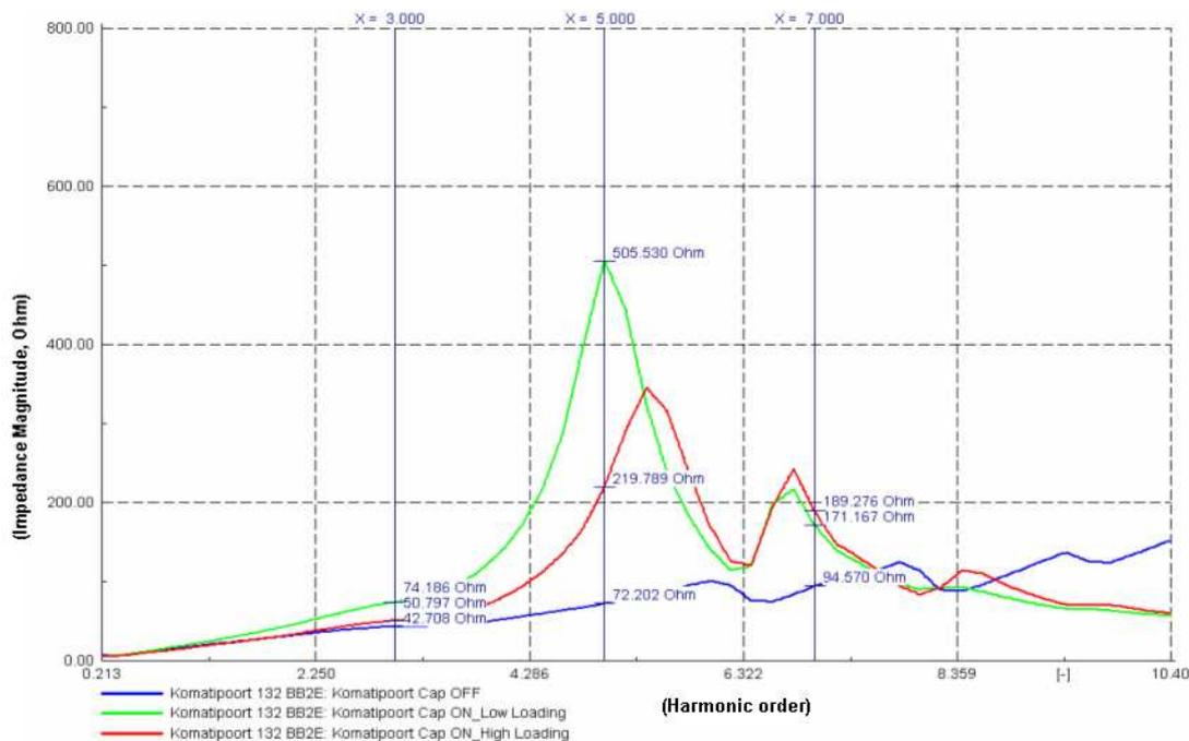
Figure 3.23: Komatipoort 132kV busbar harmonic impedance plots with the switching of the 40.5 MVAR shunt capacitor bank for various loading patterns.
