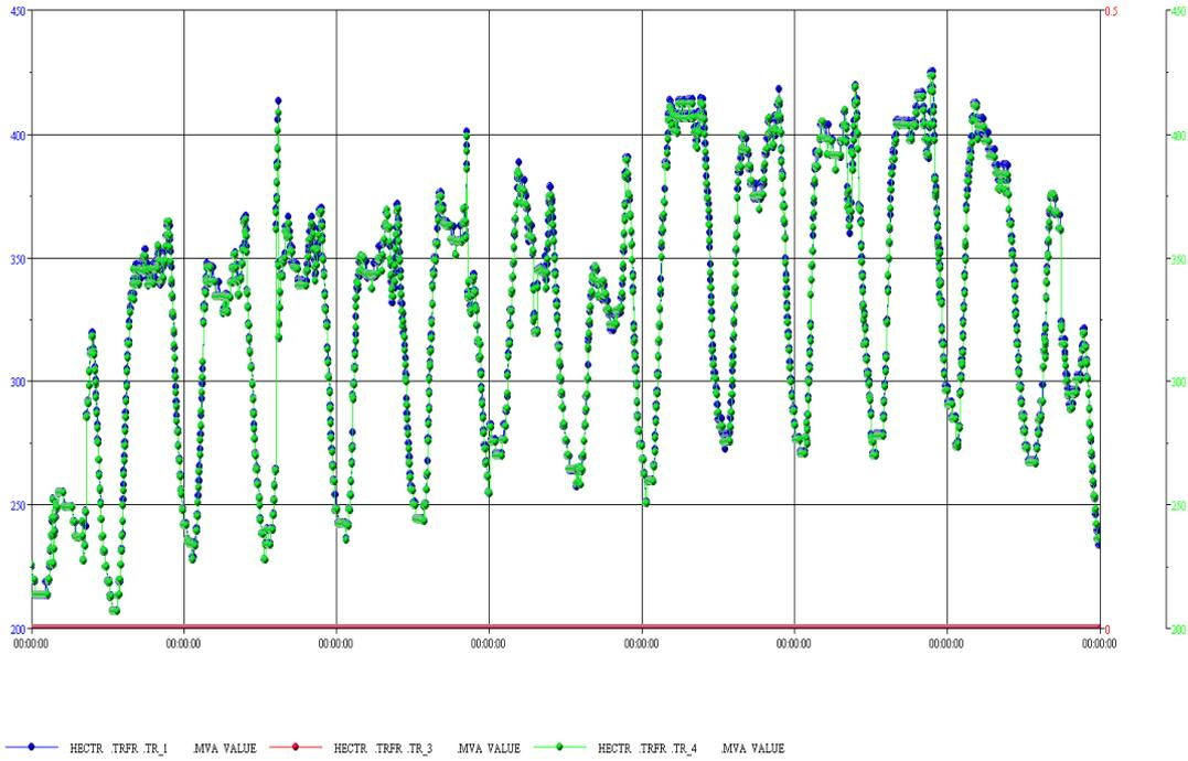
Figure 5.4: Hector 400/275kV transformer MVA loading profiles
