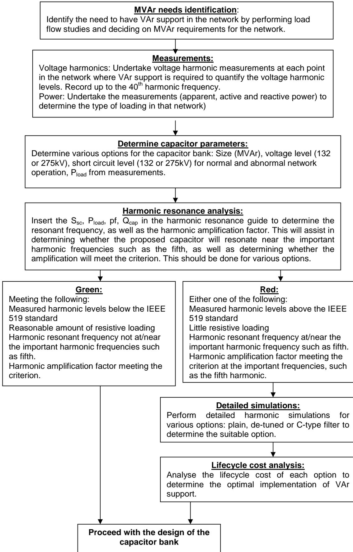
Figure 4.8: Recommended flow-chart for the assessment of harmonic resonance.
