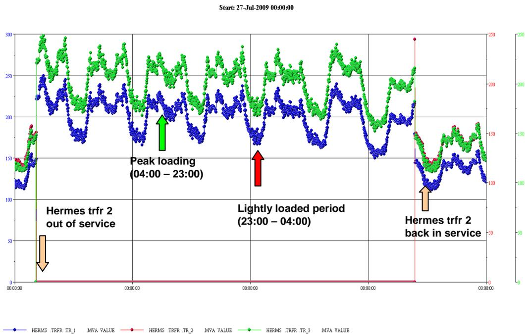
Figure 5.20: Hermes transformer MVA loading profiles
