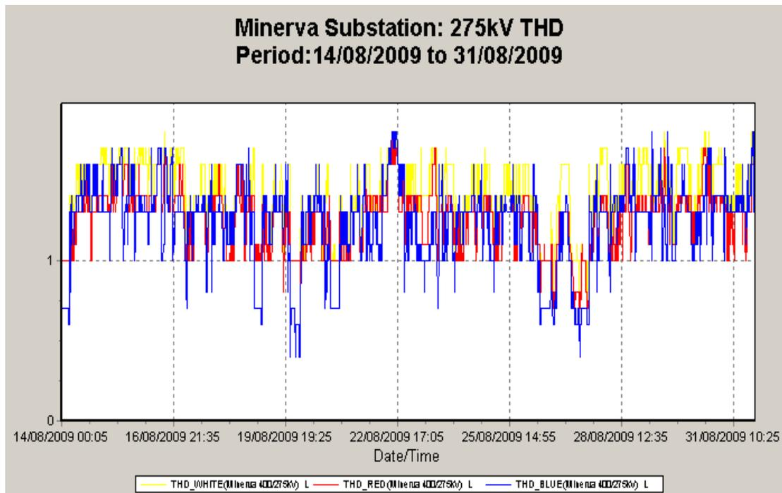
Figure 5.7: Minerva 132kV busbar THD measurements
