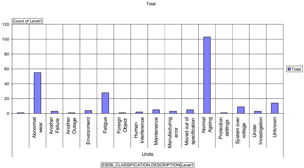
Figure 7.4: Breakdown of unit failures in HV shunt capacitor banks
