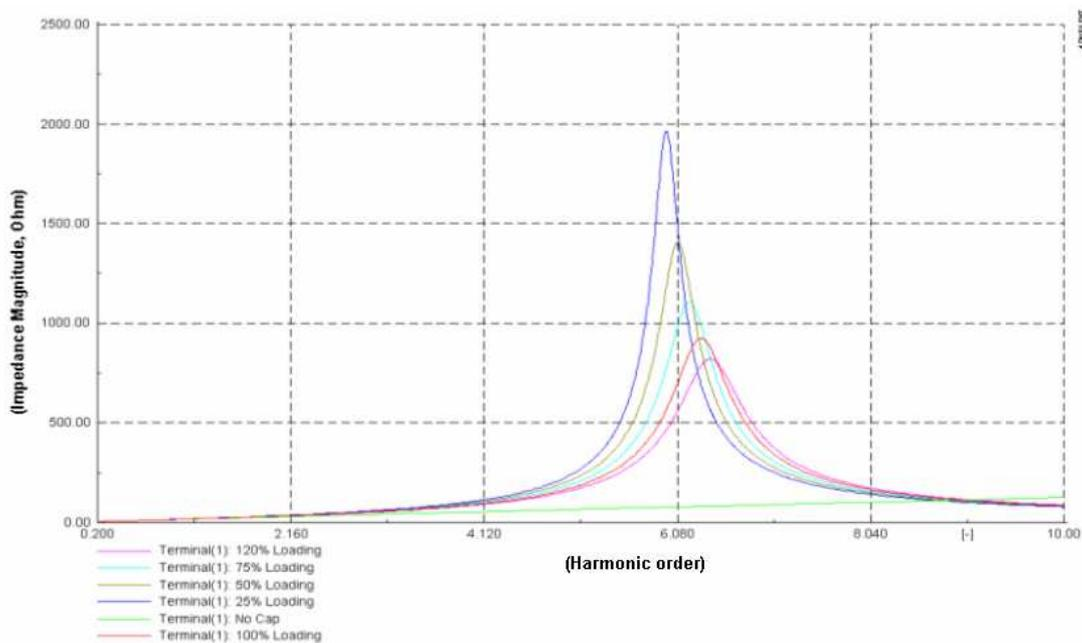
Figure 3.12: Marathon 275kV busbar harmonic impedance plots for different loading patterns.
