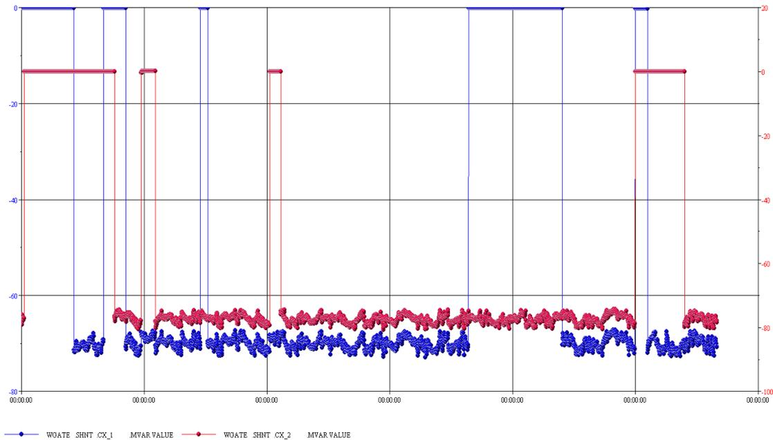
Figure 5.13: Westgate 2x72 MVar shunt capacitor bank MVar profiles
