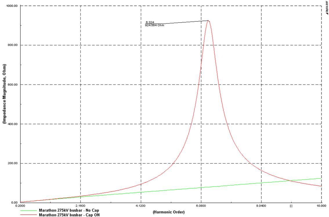
Figure 3.9: Marathon 275kV busbar harmonic impedance plots
