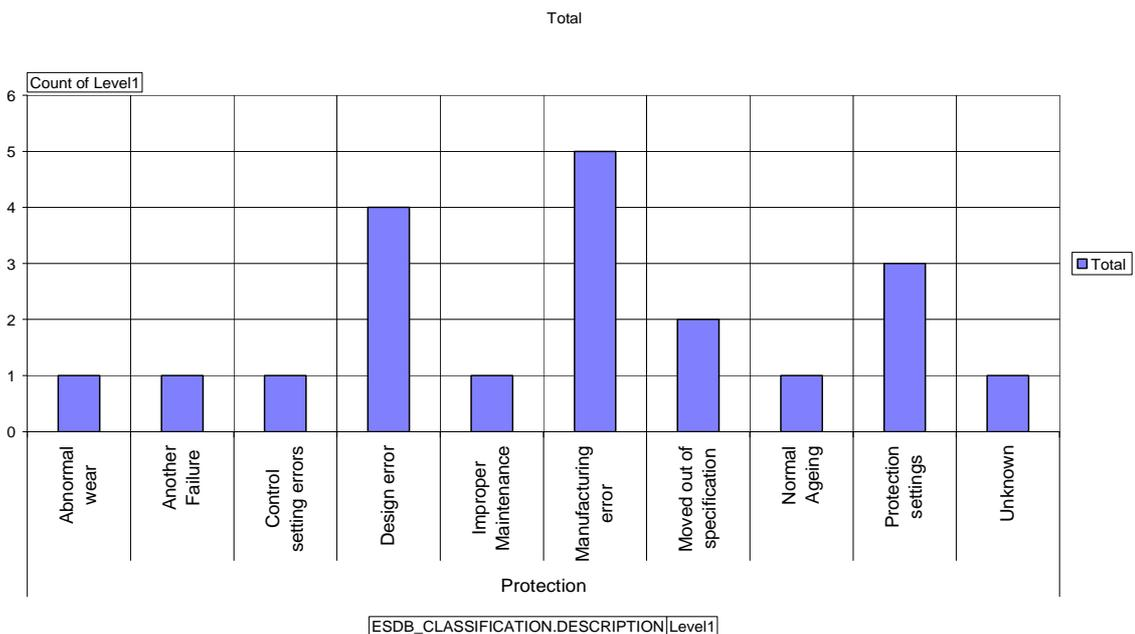
Figure 7.5: Breakdown of protection related failures in HV shunt capacitor banks
