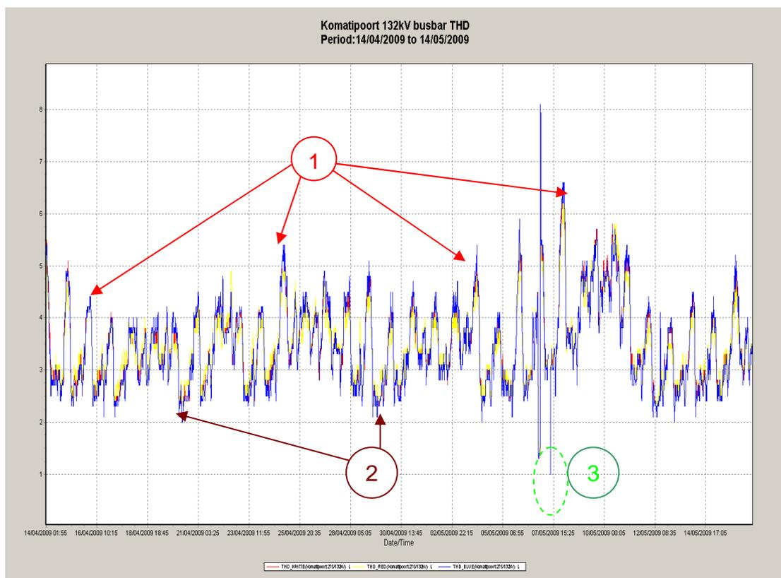
Figure 3.19: Komatipoort 132kV bus THD measurements
