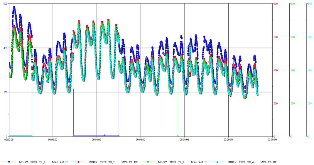
Figure 5.9: Minerva 400/275kV transformer MVA loading profiles
