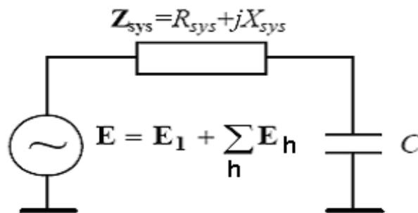
Figure 4.4: Equivalent system with capacitor to be installed
