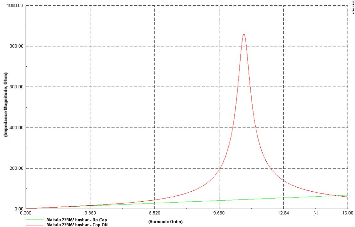
Figure 3.11: Makalu 275kV busbar harmonic impedance plots
