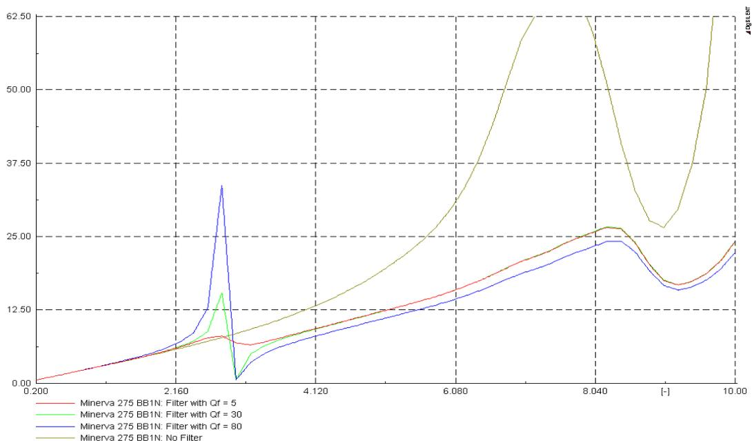
Figure 8.2: Harmonic impedance plots for the installation of a 275kV 150 MVar C-type filter with various Q factors.
