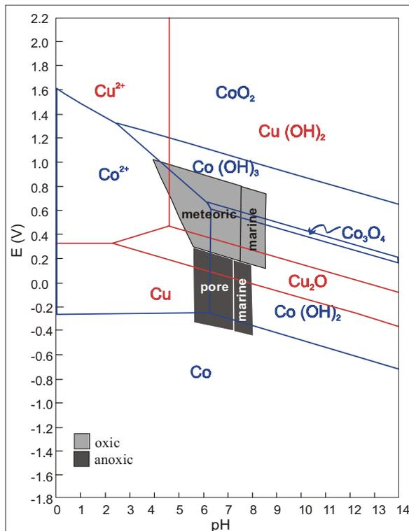
Figure 1: Potential - pH diagram for Cu and Co in the system Cu-Co-H<sub>2</sub>O at 25°C (after de Zoubov et al., 1980, and Deltombe, 1980).
