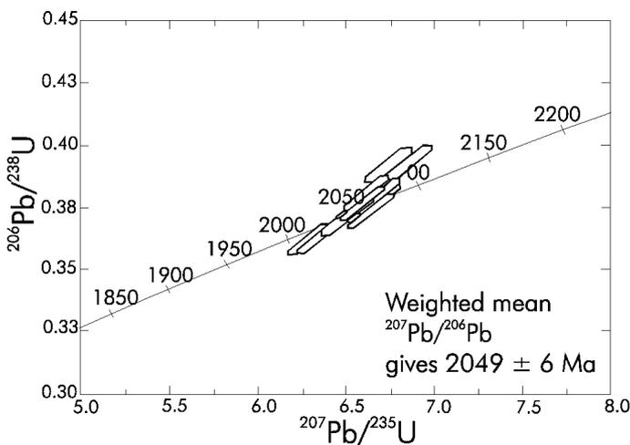
Figure 3: Concordia diagram of the Mkushi gneiss.
