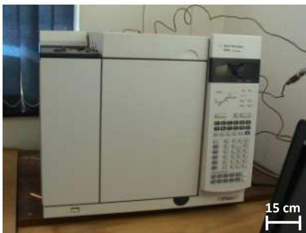
**Figure 12: Agilent 7890A GC- FID system**
