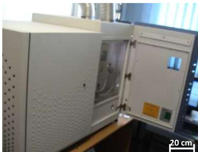
**Figure 12: ICP- OES instrument**
