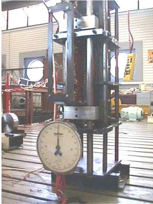
Figure 8.4: AC test with the scale attached between the secondary and the floor of the test bed
