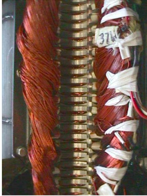
Figure 5.6: A close-up of the motor windings.
