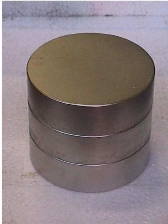
Figure 5.8: The magnet length,  $y$ , is made up of three individual magnets
