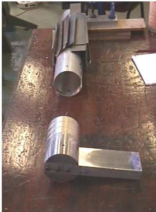
Figure 5.9: Construction of the secondary section for the buried magnet arrangement
