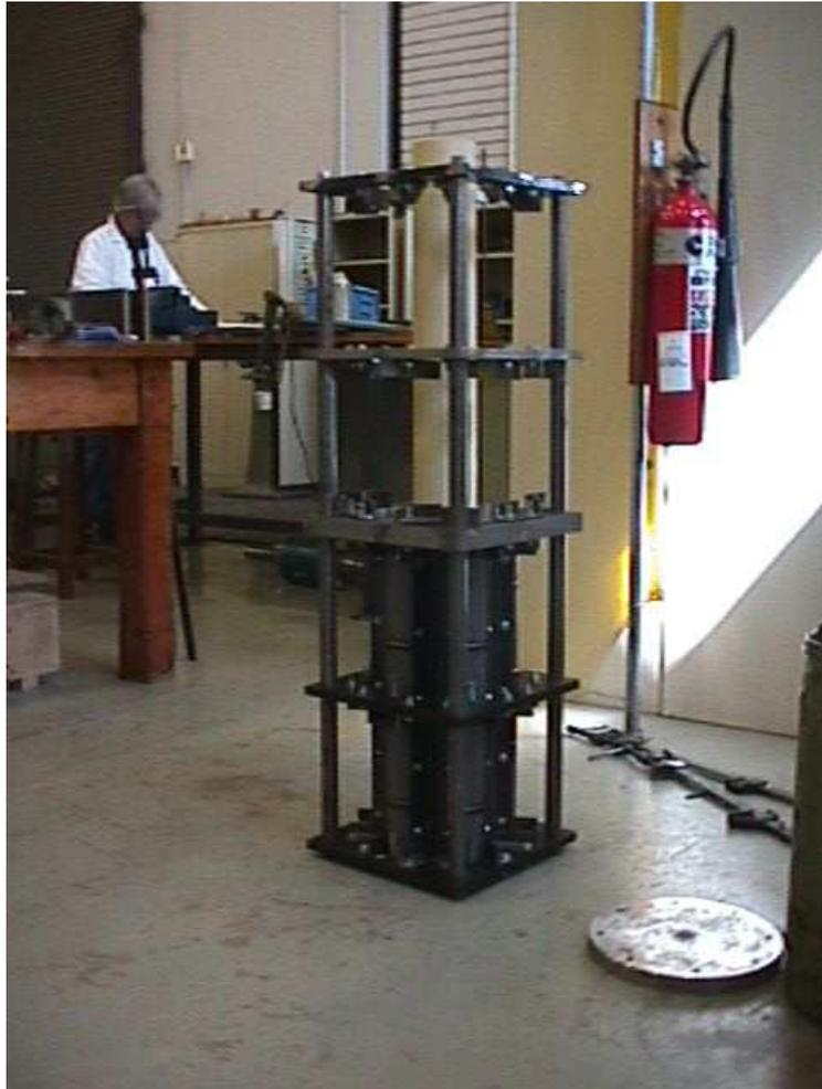
Figure 5.1: The frame of the motor with primary sections only in the bottom half.
