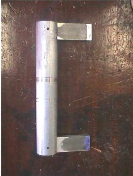
Figure 5.10: The completed secondary section for the buried magnet arrangement
