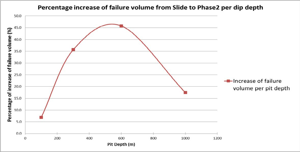
**Figure 5-24 Evaluation of failure volume increase per pit depth from Slide to Phase2**
