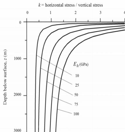
**Figure 2-2 K ratio for different deformation moduli values (Sheory, 1994)**
