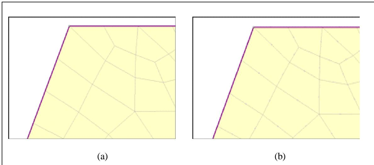
**Figure 3-3 Quadrilateral mesh elements of (a) four nodes and (b) eight nodes**
