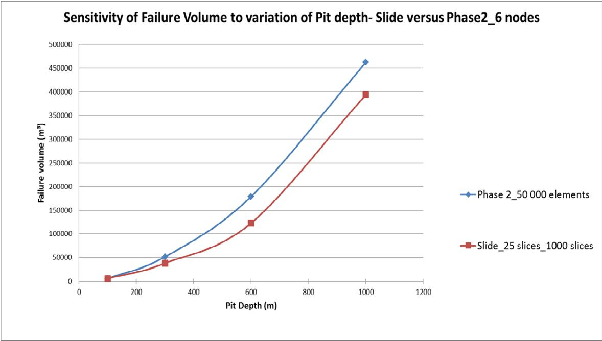
**Figure 5-23 Comparison of LE and NM failure volume sensitivities to deepening of the pit**
