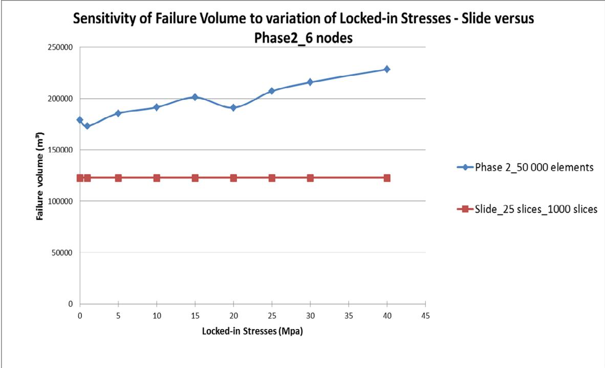
**Figure 5-31 Comparison of LE and NM failure volume sensitivities to variation of LIS**
