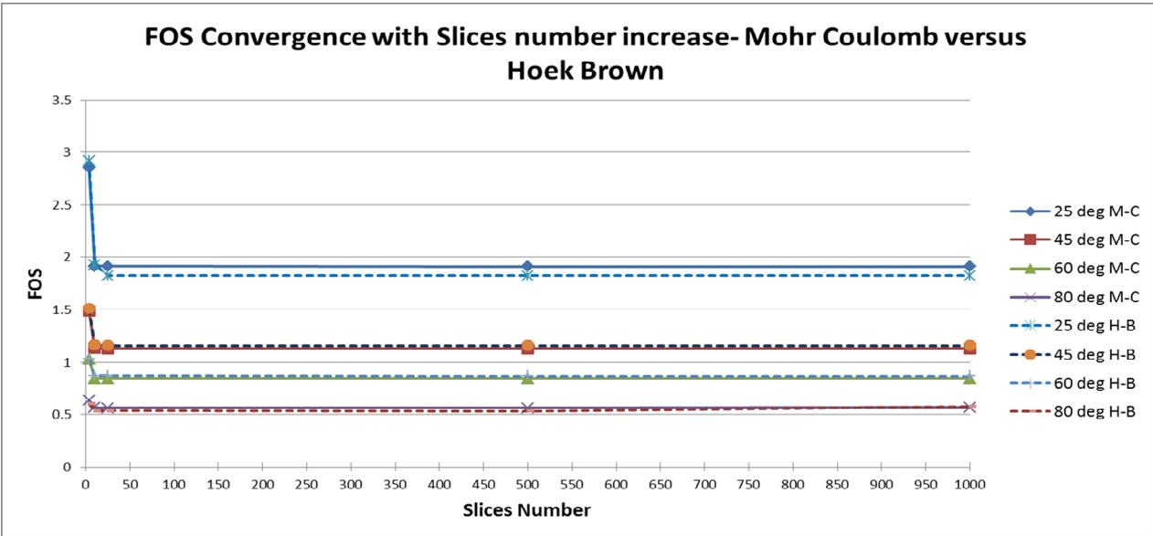
**Figure 5-1 FOS Comparisons for increases in slope angle and number of slices - Mohr Coulomb versus Hoek Brown**
