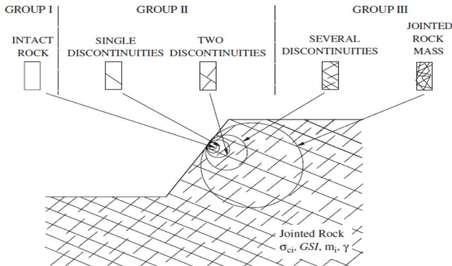
**Figure 2-10 Ranges definition of Hoek-Brown application for slope stability problems**
