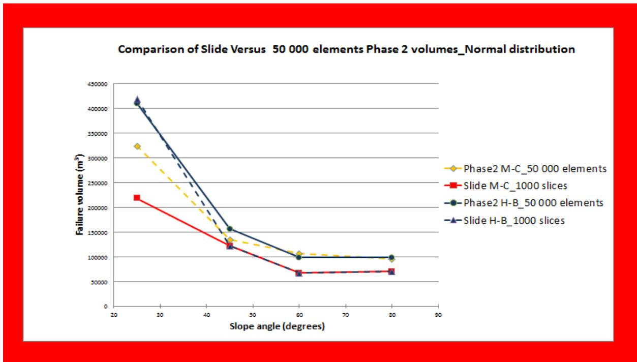
**Figure 5-20 Base case model of comparison of LE and NM failure volumes**
