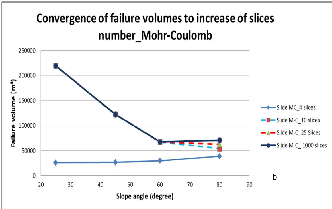
**Figure 5-6 Comparisons of failure volumes with increase in number of slices**
