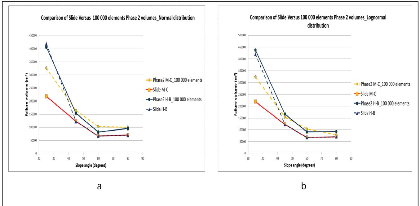
**Figure 5-19 Comparison of Slide and Phase2 failure volumes with increase of slope angle\_ case of 100 000 mesh elements**
