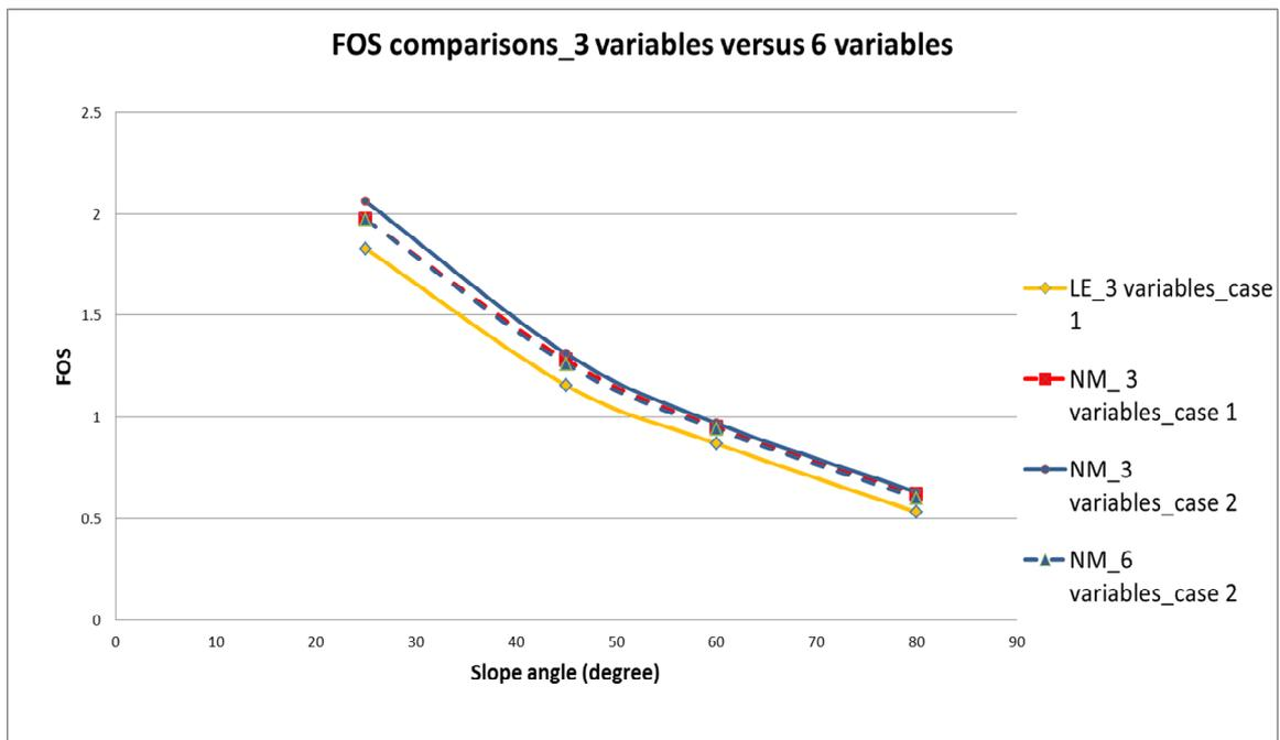
Figure 5-37 Impacts of 3 variables and 6 variables on slope stability
