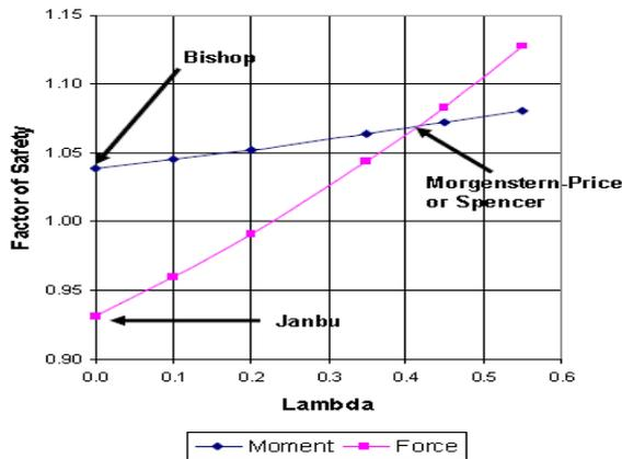
**Figure 2-7 GLE Factors of Safety with dependence on Lambda (Krahn, 2004)**
