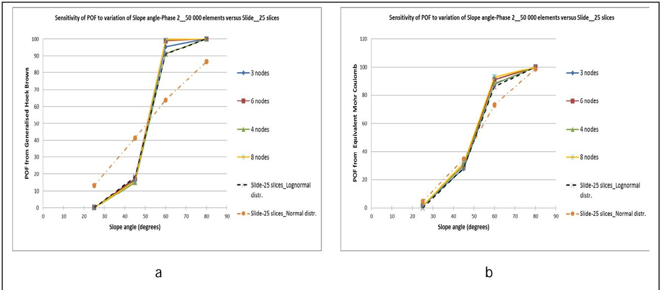
**Figure 5-14 POF Sensitivity of element type to slope angle increase\_ case of 50 000 mesh elements**
