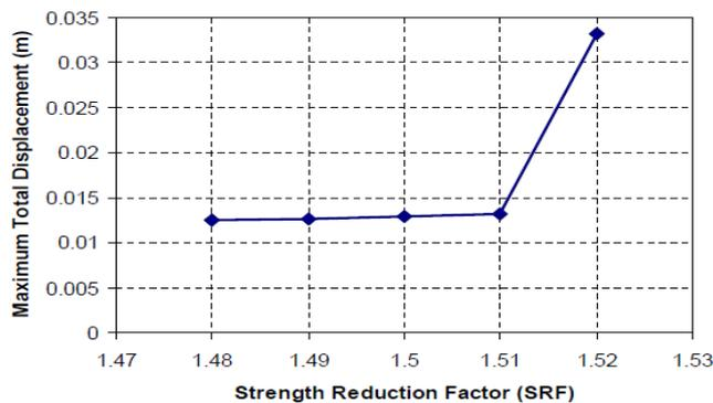
**Figure 2-12 Strength reduction factor versus maximum total displacement**
