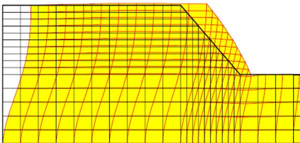
**Figure 2-3 Snapshot of deformation during an earthquake, after Krahn (2004)**
