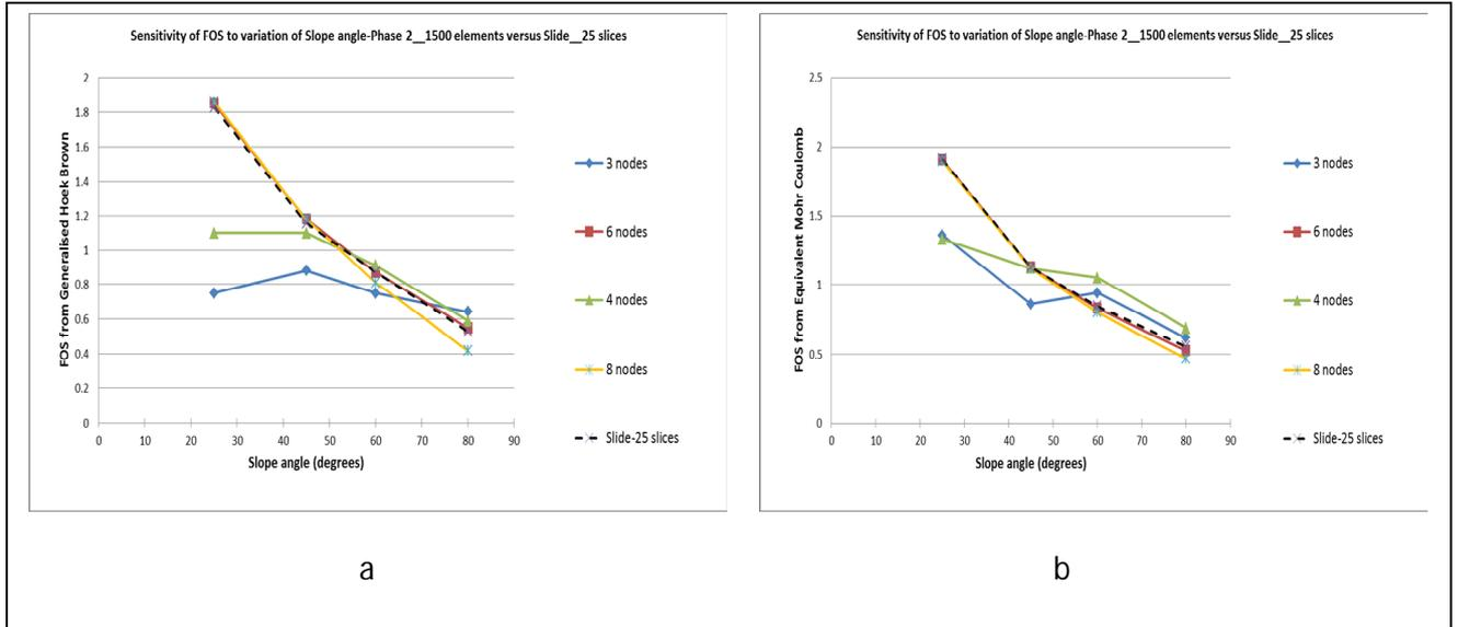
**Figure 5-9 FOS Sensitivity of element type to slope angle increase\_ case of 1500 mesh elements/ lognormal distribution**
