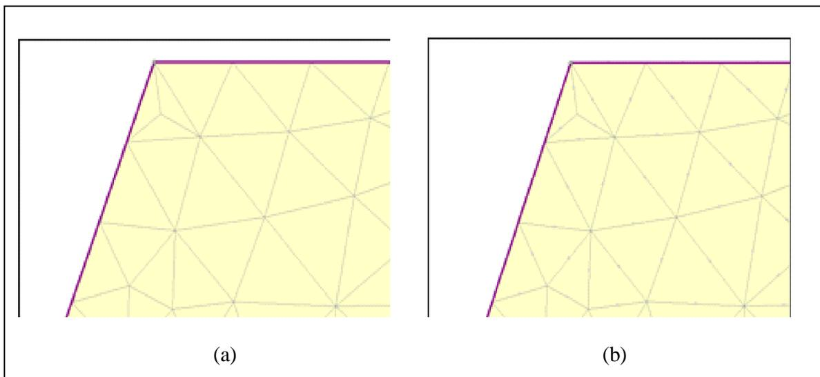
**Figure 3-2 Triangular mesh elements of (a) three nodes and (b) six nodes**
