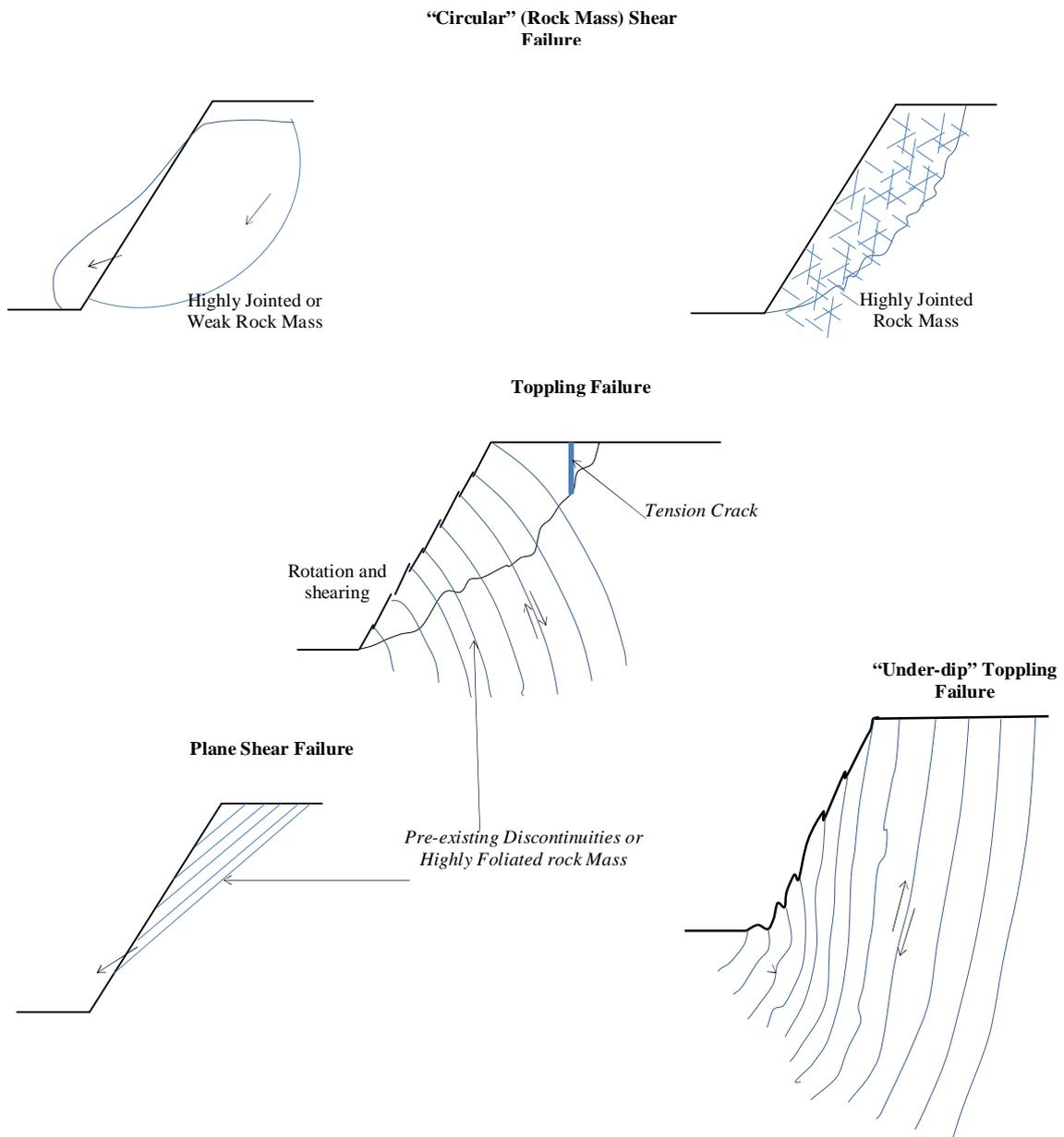
**Figure 2-6 Analysed failure modes, after Hustrulid *et al.*, (2000)**
