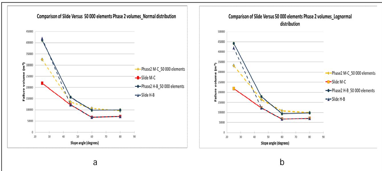
**Figure 5-18 Comparison of Slide and Phase2 failure volumes with increase of slope angle\_ case of 50 000 elements**
