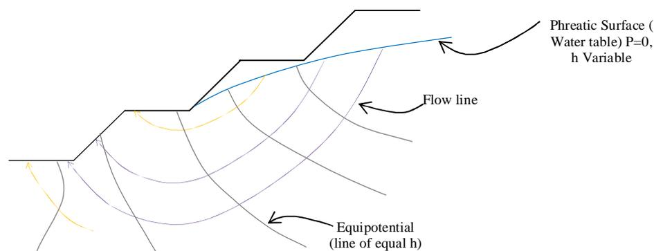
**Figure 2-5 Groundwater Flow Anatomy System in Pit Slope (Hustrulid *et al.*, 2000)**
