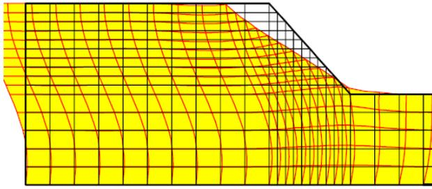
**Figure 2-4 Snapshot of backward slope deformation during an earthquake, after Krahn (2004)**
