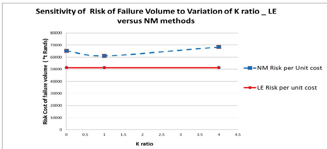
**Figure 5-28 Comparison of LE and NM risks of failure volumes to variation of K ratio**
