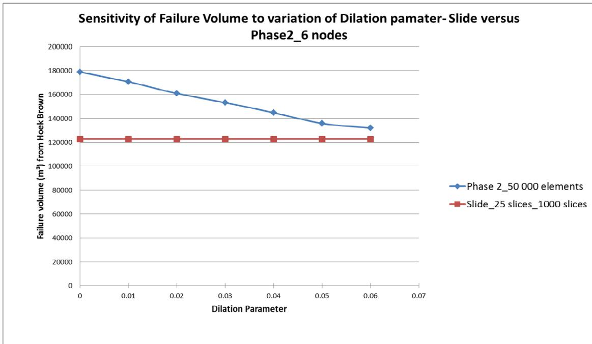
**Figure 5-35 Comparison of LE and NM failure volume sensitivity to variation of dilation parameter**
