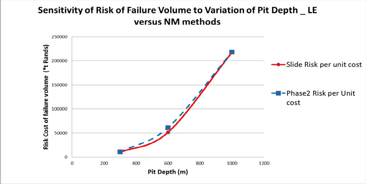
**Figure 5-25 Comparison of LE and NM risks of failure volumes to variation of pit depth**
