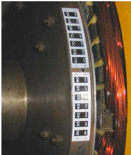
Figure 5: Holes in rotor backiron for insertion of temperature probes.
