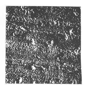
Fig. 11. Dentine aspect of fractured Cosmic experimental bond on polished dentine surface pretreated with Cosmic Bond. Bond strength 8,7 N mm<sup>-2</sup>. SEM X 2000.
