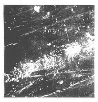
Fig. 7. Adhesive aspect of fractured bond shown in Fig. 6. SEM X 2000.
