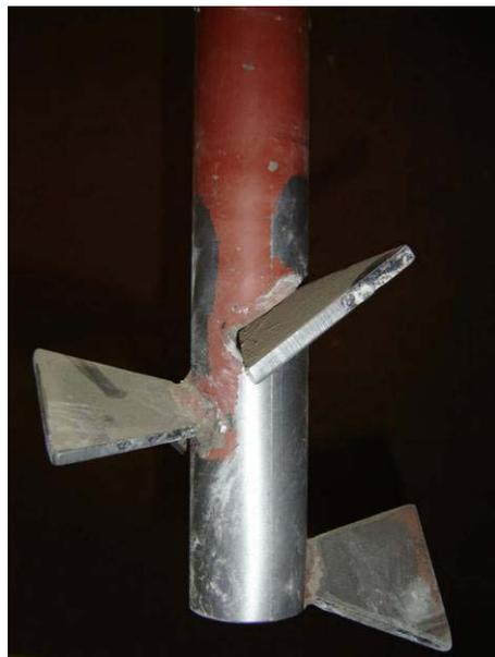
**Figure 4.1:** Interrupted helical impeller for the Tattersall Two Point Tester
