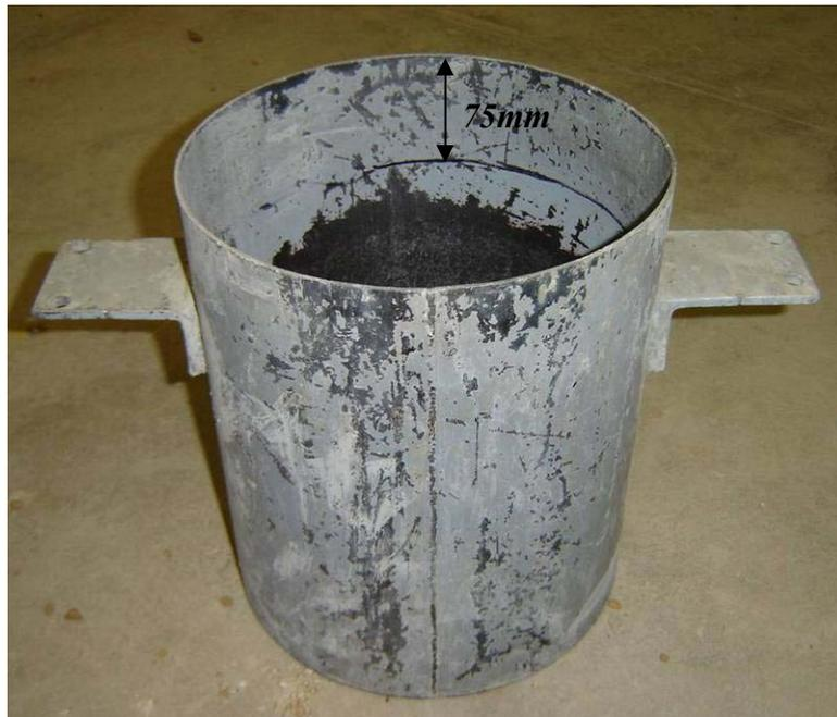
**Figure 4.3:** Sample holder showing the filling mark
