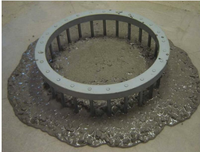
**Figure 4.11:** The J-Ring test
