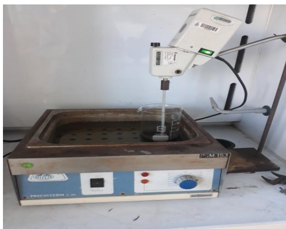
Figure 5: Extraction experiment using water bath and electrical stirrer.
