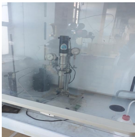
Figure 8: Experimental gas / liquid reactor autoclave connected to flow meter
