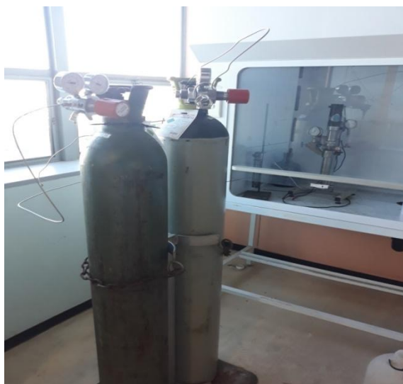
Figure 7: Gas tanks of carbon dioxide under pressure surmounted by a regulator
