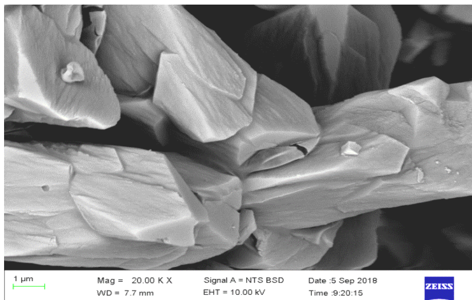
Figure 31: Calcium carbonate precipitate obtained by using \text{NH}_4\text{NO}_3 solvent after 15 minutes with an injected \text{CO}_2 pressure of 4 bars.
