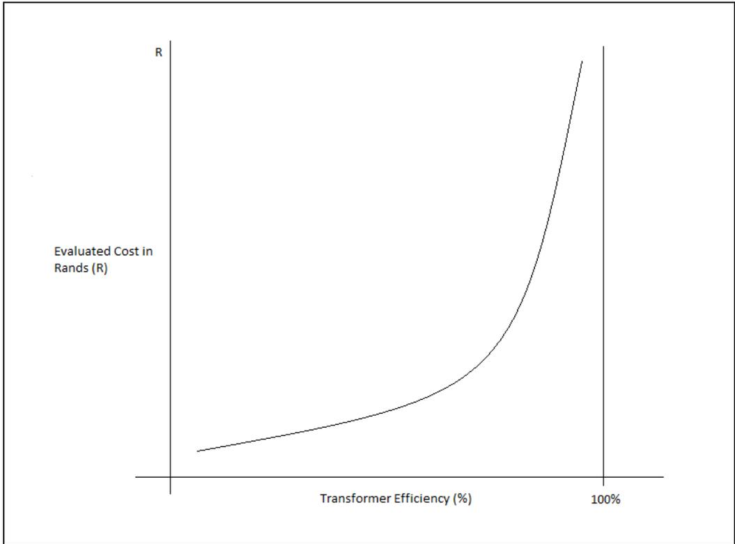
**Figure 2: Transformer cost and efficiency relationship, an increase in efficiency results in an increase in the capital cost of the transformer**
