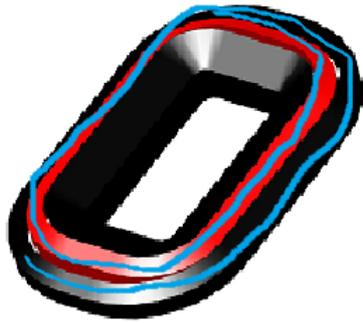
**Figure 6: Continuous magnetic flux path in the hexa-transformer**
