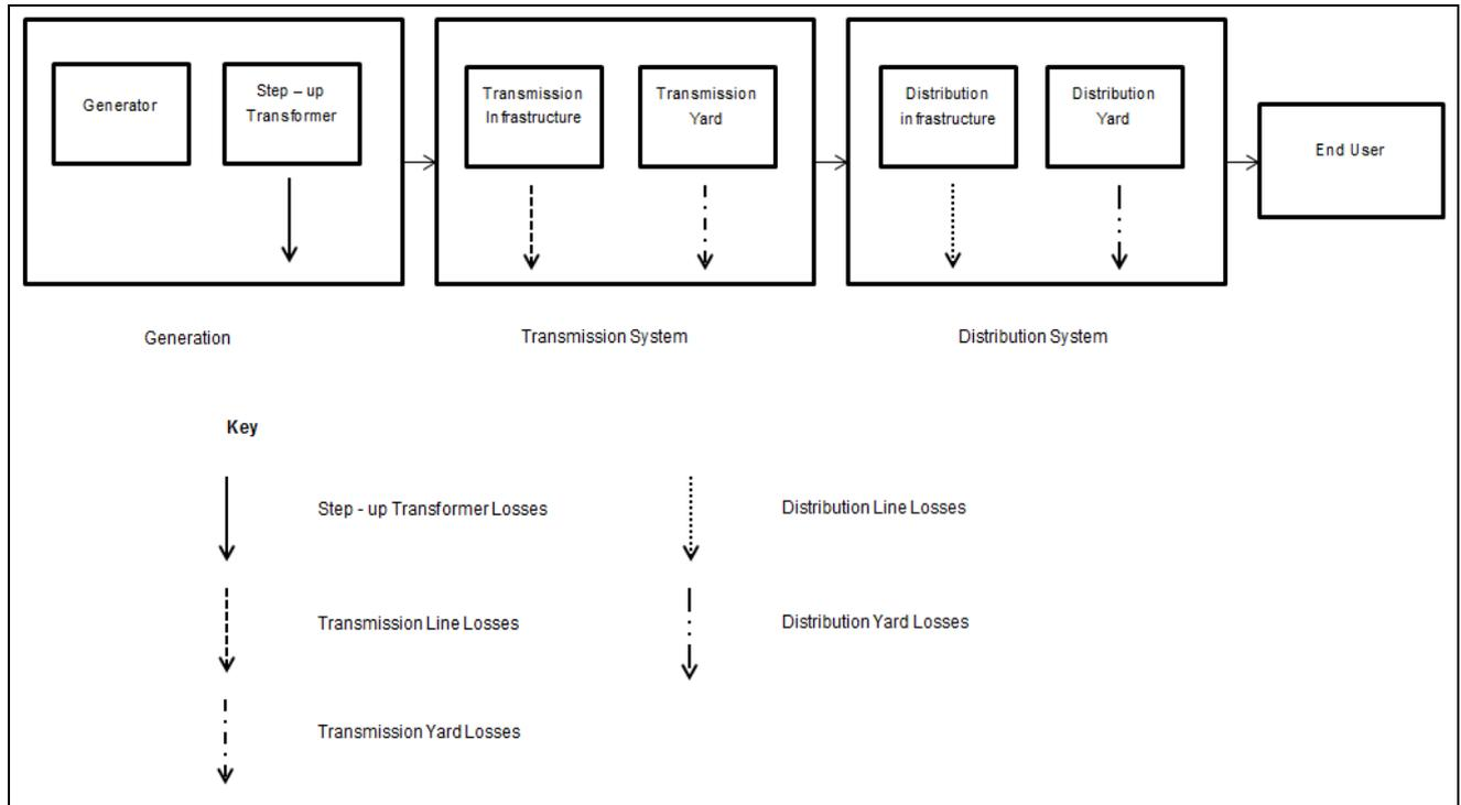
**Figure 1: Electricity distribution illustrating the flow of electricity from generation to the consumer**
