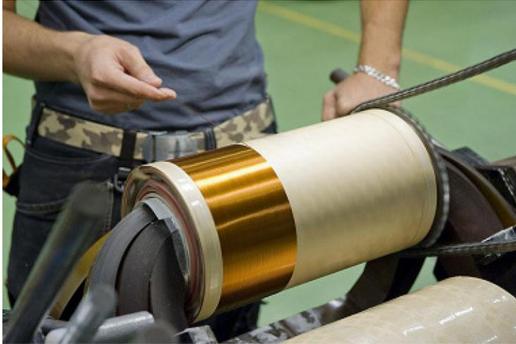
**Figure 10: High voltage winding is wound using a tube that rotates**
