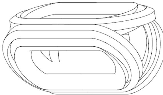
**Figure 3: The Hexa-transformer illustrating the nine rolls of steel bands**
