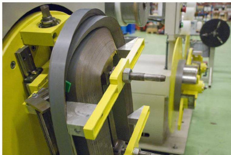
**Figure 9: Hexaformer core is wound using continuous electrical steel**
