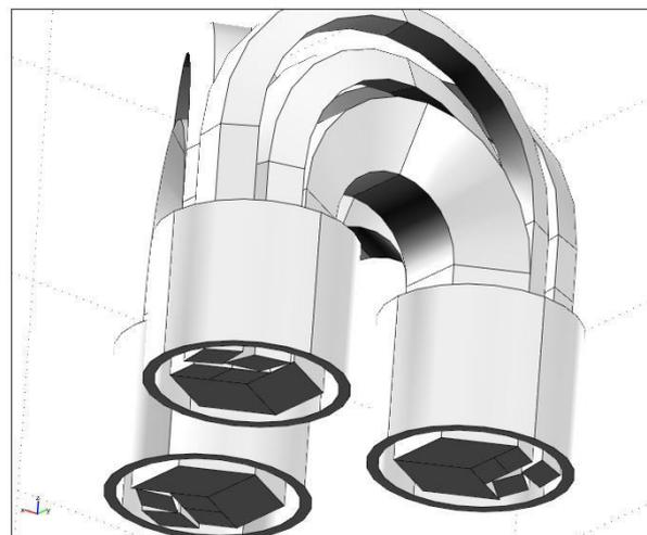
**Figure 4: Model of the hexa-transformer illustrating cross section legs**
