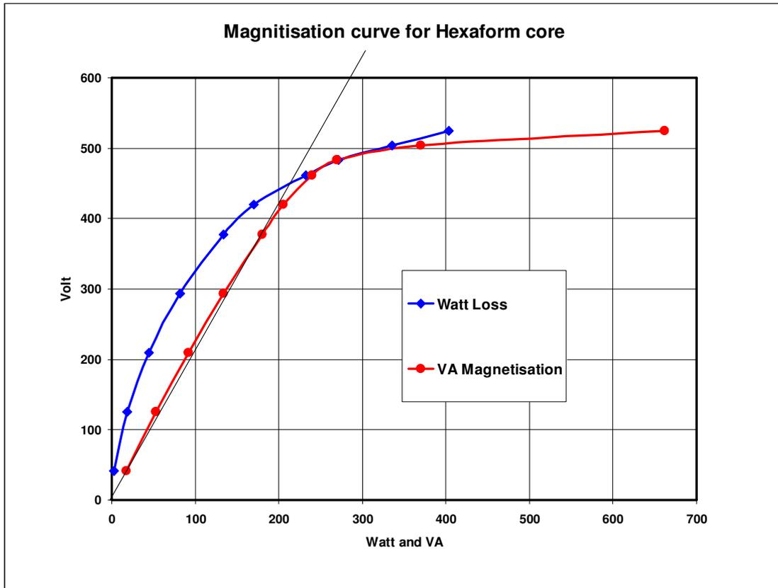
Figure 12: Eskom/Powertech magnetization curve of the hexa-transformer core
