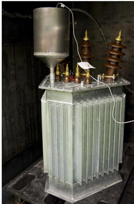
**Figure 11: Oil filling; the transformer is filled with oil under a vacuum**
