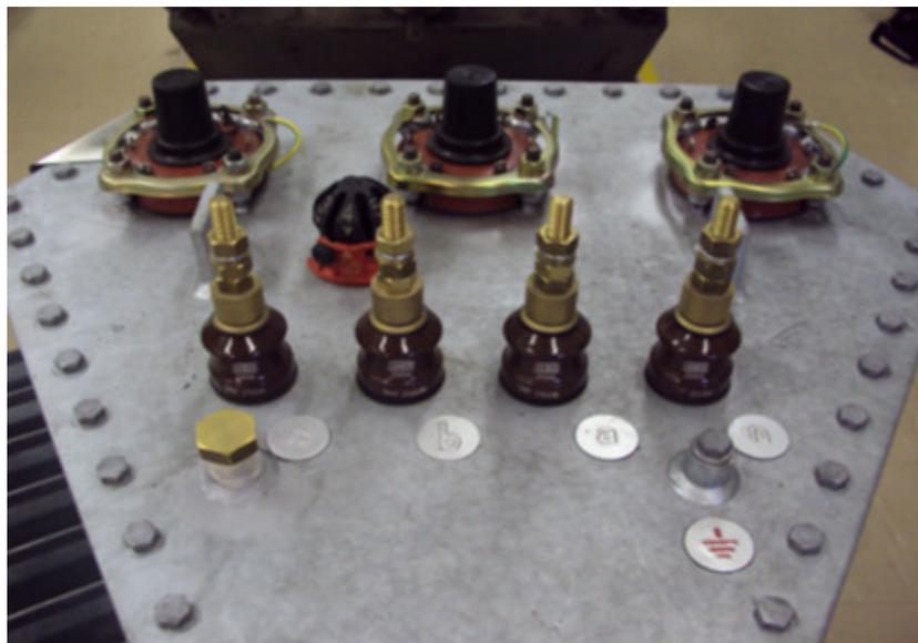
**Figure 15: Porcelain bushings are attached to lid of the hexa-transformer unit**
