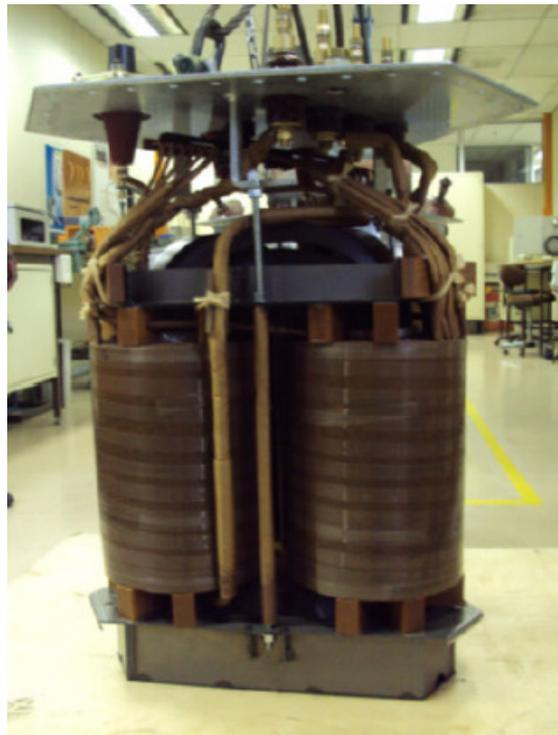
**Figure 19: Hexa-transformer unit removed from tank**
