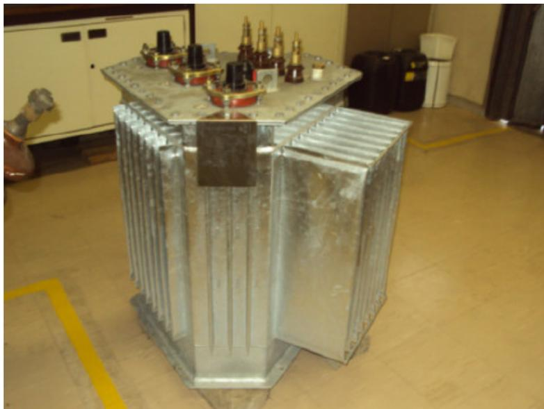
**Figure 14: Hexa-transformer complete unit**
