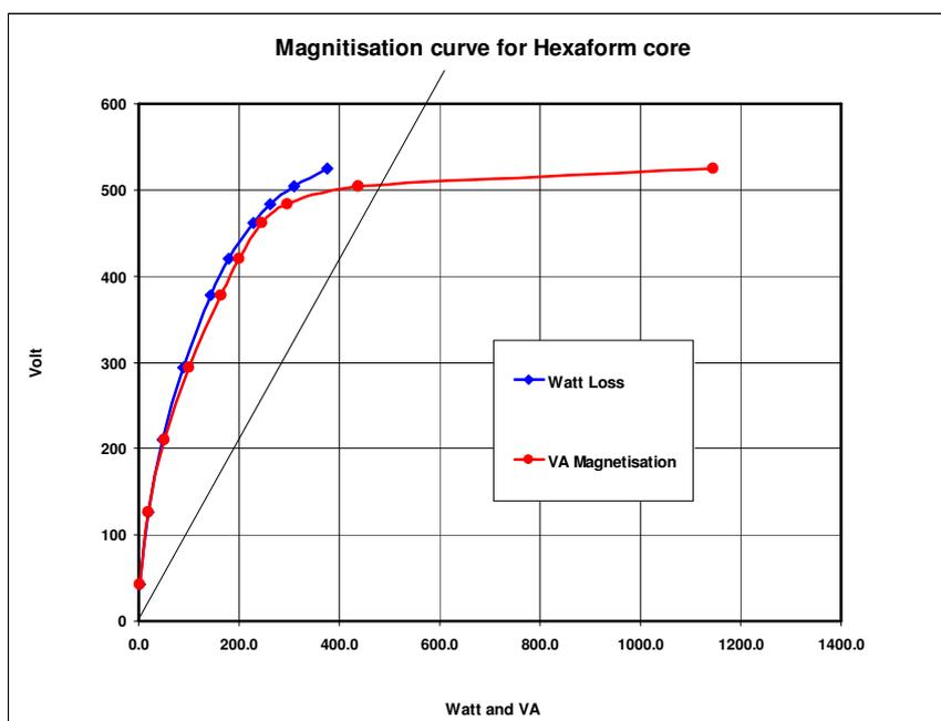
**Figure 13: Hexaformer AB magnetization curve of the hexa-transformer core**
