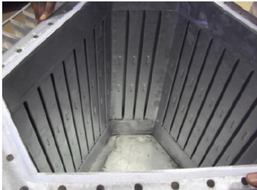
**Figure 17: Tank Sealing Material of the hexa-transformer unit**
