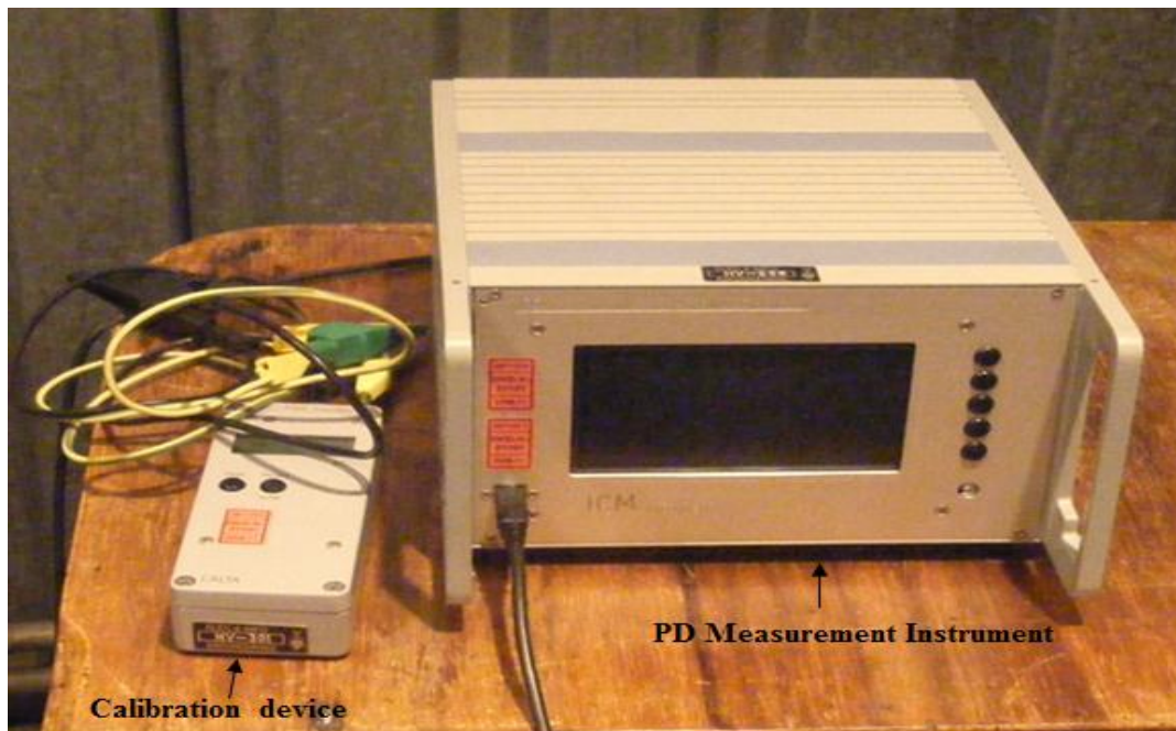
Figure 5-6: A picture of the ICM Compact PD measuring instrument
