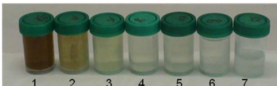
**Figure 5.77:** Aliquots collected after different leaching times.
