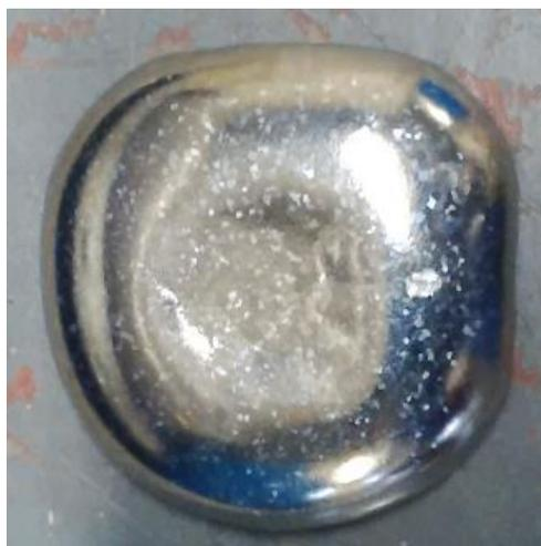
Figure 3.3: Type 304L stainless steel ingot alloyed with 1 wt% Ru.
