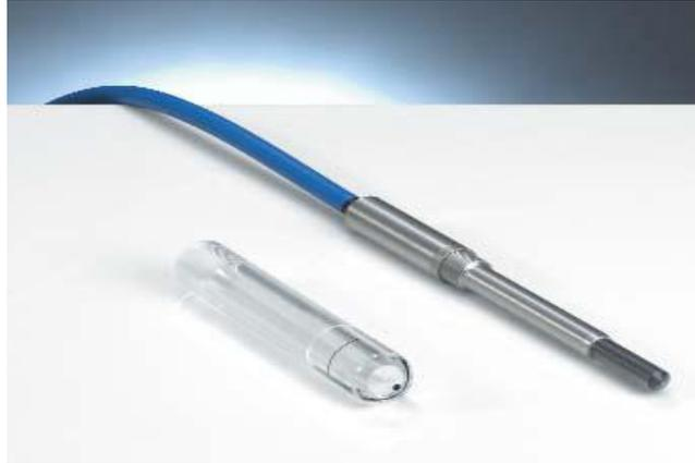
**Figure 4.4:** A PTW 30013 waterproof therapy chamber for absolute dosimetry in high-energy photon, electron and proton beams with sensitive volume of 0.6 cm<sup>3</sup>, vented to air (54).
