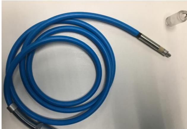
**Figure 4.2:** An ultra small-sized pinpoint therapy chamber with 3 dimensional characteristics for dosimetry in high-energy photon beams.
