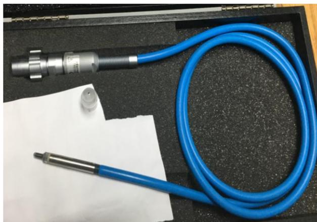
**Figure 4.1:** The small-sized PTW 31006 pinpoint 0.015 cm<sup>3</sup> therapy chamber for dosimetry in high-energy photon beams that was used in this study.
