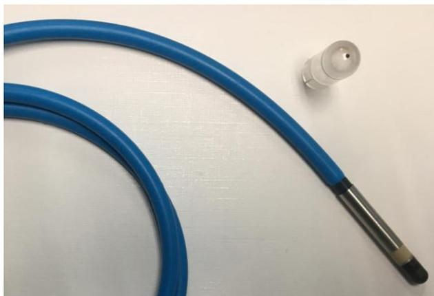
**Figure 4.3:** A PTW 31010 semiflex 0.125 cm<sup>3</sup> standard therapy chamber for scanning systems and for relative and absolute dosimetry.
