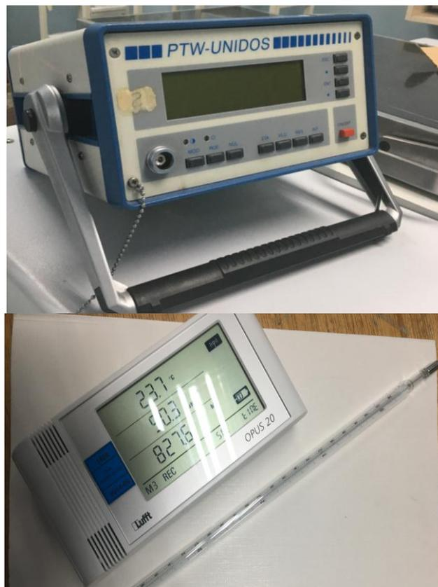
**Figure 4.6:** A PTW Unidos electrometer that was used to measure the charge, a Lufft Opus 20 temperature, humidity, air pressure data logger device for determining the pressure and the temperature in the room, and the mercury thermometer that was used for measuring the water temperature in the water tank. All these devices were used for measurements during the experiment.
