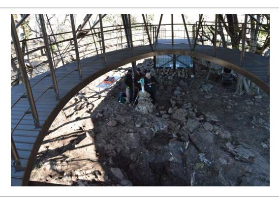
Figure 1: The use of conventional coordinate capture methods during excavations at Malapa Cave, Cradle of Humankind. The excavators are using a Nikon NPR-352 total station mounted on a known-position survey point to record the position of fossil material recovered during the excavation process. Site coordinates (x, y and z) are converted to geo-reference coordinates (easting, northing and height above sea level in the WGS 84 map reference system) by the total station.
