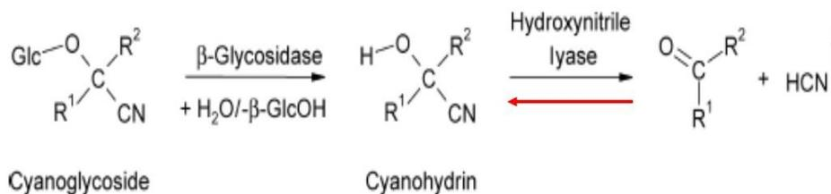
**Figure 5. The process of cyanogenesis catalysed by hydroxynitrile lyases.** Cyanogenic glycosides are hydrolysed by  $\beta$ - glucosidase enzymes to yield a chiral cyanohydrin. The cyanohydrin is cleaved by hydroxynitrile lyases into the corresponding carbonyl compound and gaseous hydrogen cyanide. The reverse reaction is desirable in industry (Effenberger *et al.*, 2007).
