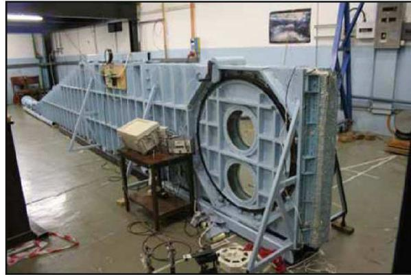
Figure 2.11: Shock tube used by Skews et al. (2009).
