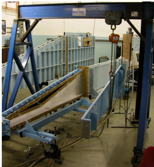
Figure 5.4: Replacement of a ramp section in the diverging section.
