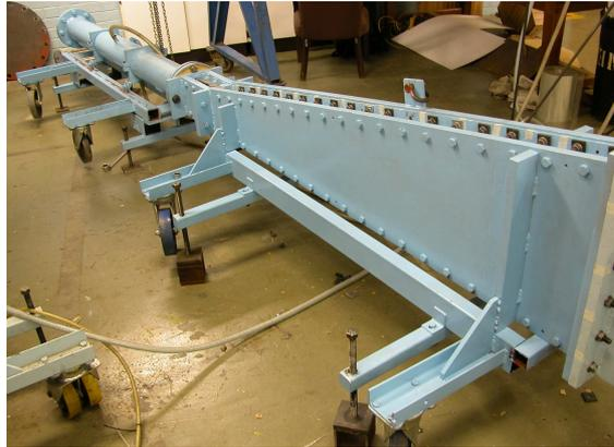
Figure 5.3: Newly manufactured diverging section and driver.
