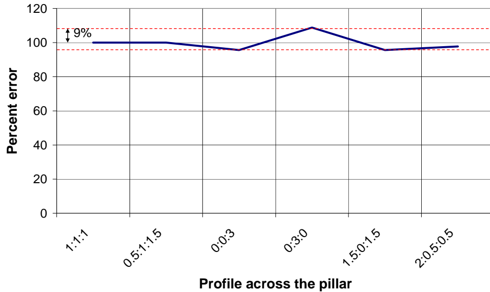
Figure G 26 Synopsis of potential errors associated with stress profiles across Impala P2
