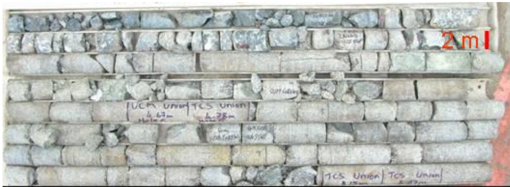
Figure E 15 Core from the footwall extensometer
