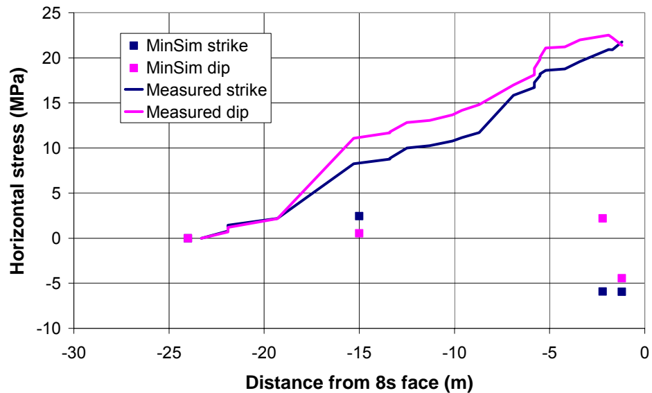
Figure E 42 Horizontal stress change 4.2 m above Pillar 2 in Borehole CSIRO1. Negative face positions are behind the cell
