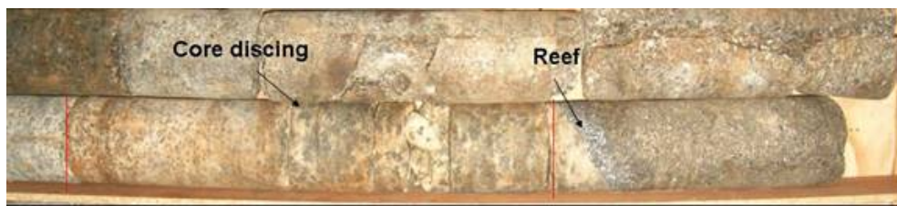
Figure E 57 Core discing observed in the F/W anorthosites
