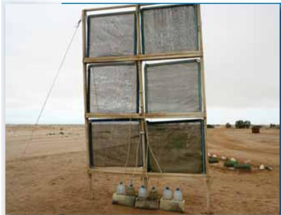
Figure 2.6 Fog harvesting equipment (Source: University of Namibia website, 2009)
