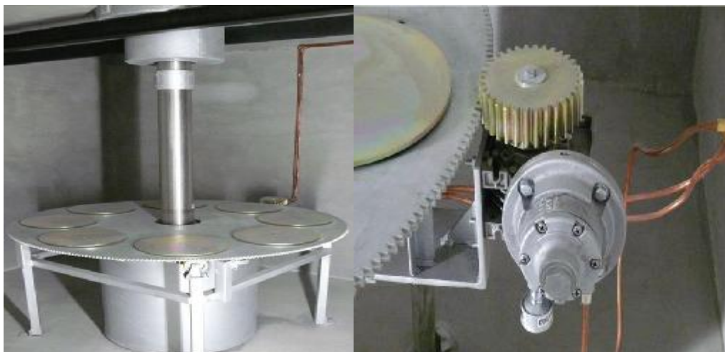
Figure 3.2: Left hand side: The main turntable with 8 mini-turntables. Right hand side: Electrical motor driving the turntable.
