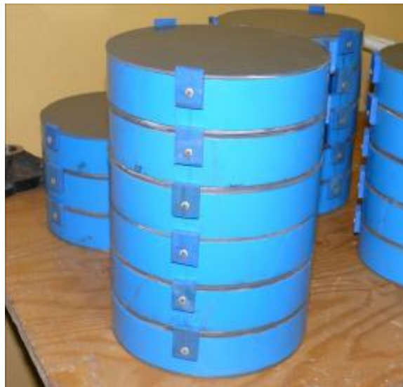
Figure 3.3: An orderly pile of six cylindrical containers used for insects irradiation.
