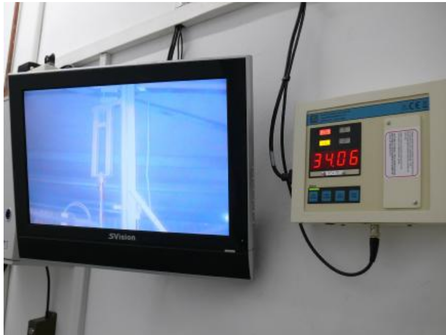
Figure 3.7: Television and area detector monitor which displays the status of the source inside the irradiator chamber and the radiation monitor used to display the dose rate at the detector position.
