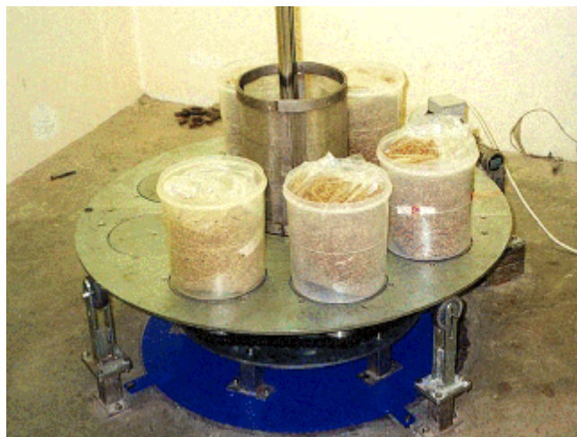
Figure 3.8: A circular main turntable with the cylindrical containers filled with insects on top of the mini-turntables.
