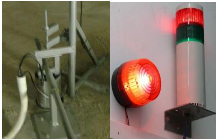
Figure 3.6: The mechanical source interlock system and strobe light-system.
