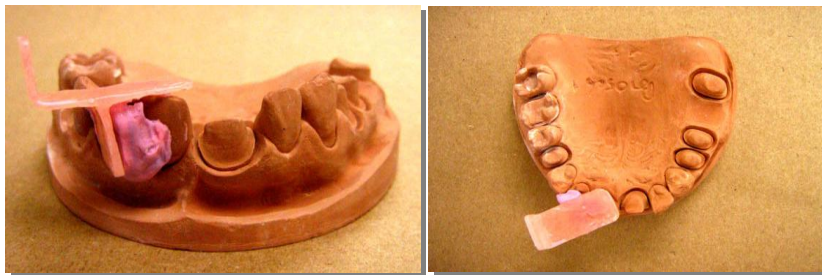
Fig 3.13 Set-up of stabilising (acrylic) device with lab putty to simulate quadrants 2 and 4
