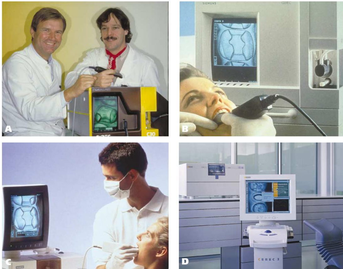
Fig 1.3 Evolution of CEREC hardware. A. 1985: the CEREC 1 prototype unit, the “lemon,” with Dr. Werner Mörmann (left) and Marco Brandestini, Dr. sc. techn.ETHZ. B. 1991: CEREC 1, as modified by Siemens (Munich, Germany) with E-drive and CEREC Operating System 2.0. C. 1994: CEREC 2, with an upgraded three-dimensional camera. D. 2000: CEREC 3, with split acquisition/design and machining units (With permission-SIRONA)
