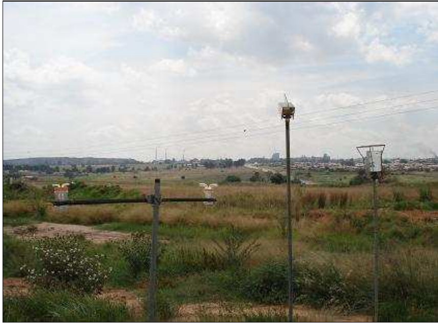
Figure 3.4: Modified WDFG, MWAC N, MWAC D and the Single Bucket Schoongezincht Mini-pit site RAMP 6
