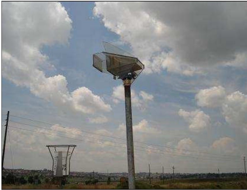
Figure 3.3: Modified WDFG Sampler and the Single Bucket at Schoongezincht Mini pit Site RAMP 6
