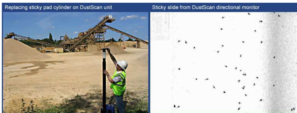
Figure 2.8 Photograph showing sticky pad cylinder and slide on DustScan unit. After Goodquarry (2004)
