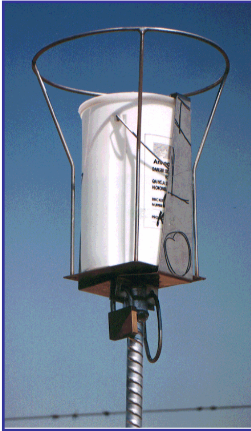
Figure 3.6: Single Bucket monitoring unit, showing sampling bucket with bird ring and Security clamp
