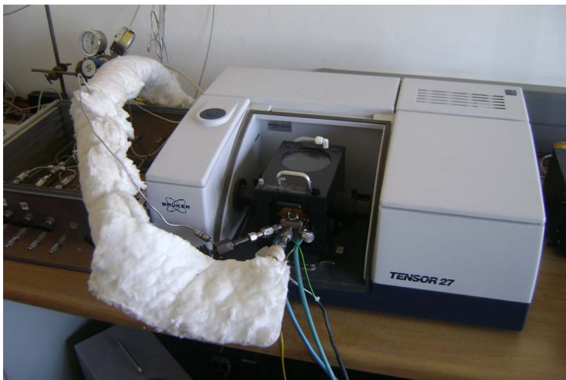
Figure 3.4 Gas manifold for the introduction of gases into the DRIFTS cell
