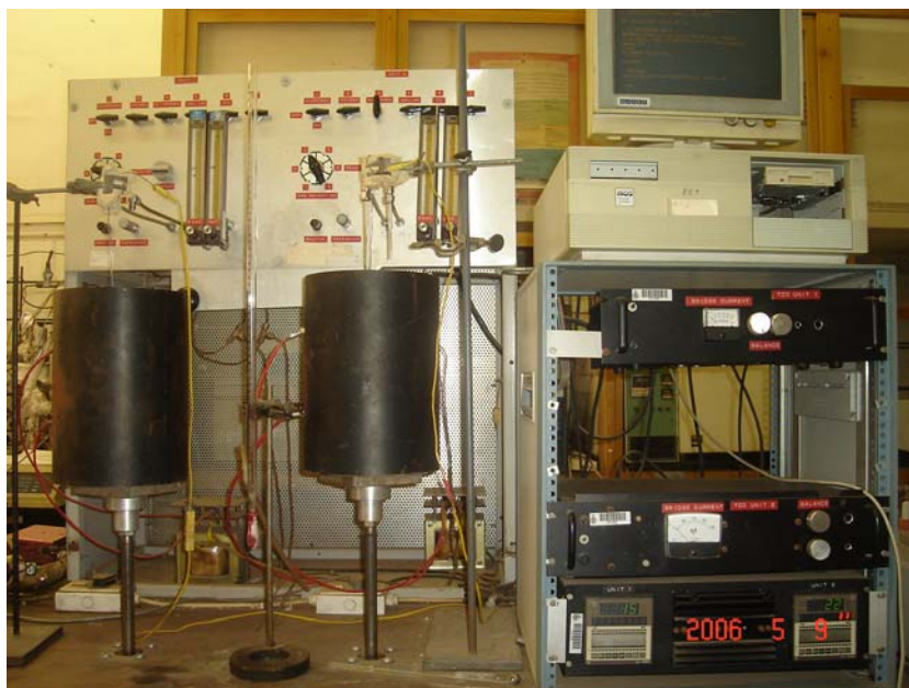
Figure 3.2 Experimental set-up for TPR measurements
