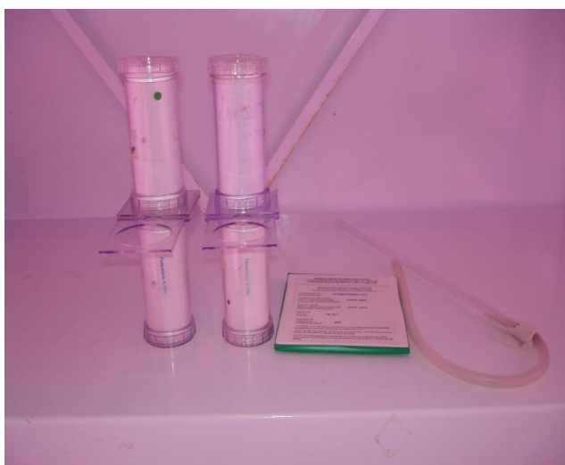
Figure A.4: WHO test kits for testing adult anopheline susceptibility to insecticide, insecticide treated papers and an aspirator.
