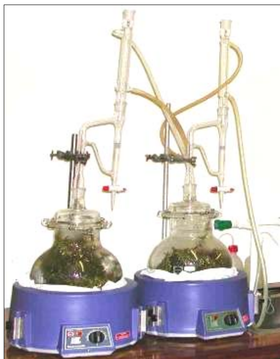
Figure 2.1 Clevenger apparatus used for the isolation of the essential oils.
