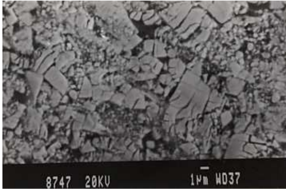
Figure 4.20: SEM micrograph of a WC-12wt%Co specimen worn for approximately 120 seconds under 2.16N load in “No debris” wear condition showing severely cracked WC grains, WC grain fragments and pits. The micrograph was taken along the edge of a groove and represents typical wear of the “No debris” condition.
