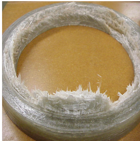
Figure 7.15: Failed stub flange
