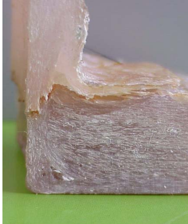
Figure 7.20: Cracks across the entire hub flange
