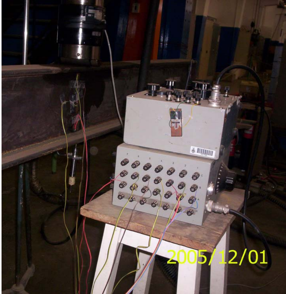
Figure 3.12 – Connecting wires to strain gauge reader
