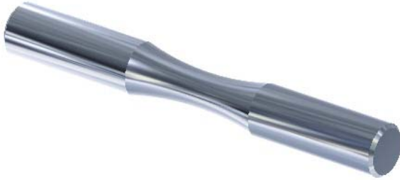
Figure 2.2 – A polished laboratory specimen
