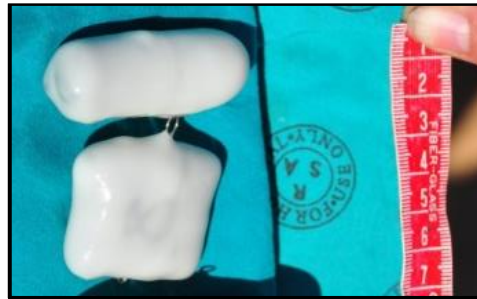
Figure 2.9: Two different data loggers were implanted into the animals: a) miniature temperature-sensitive data loggers (DST centi-T, Star-Oddi, Iceland) covered in wax (top); (b) motion-sensitive loggers (ADXL345, Sigma Delta Technologies, Australia) covered in wax (bottom) and were tethered to the abdominal muscle wall. A measuring tape is added to indicate relative size. The motion-sensitive loggers were inserted into the retroperitoneal space and the motion-sensitive data loggers were tethered to the abdominal muscle wall.
