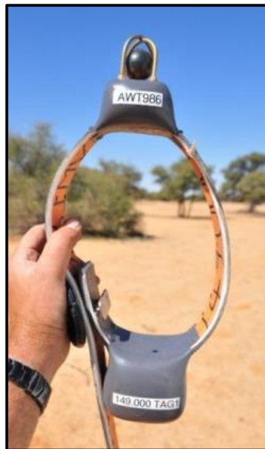
Figure 2.8: A satellite-based GPS collar (African Wildlife Tracking, Pretoria, South Africa) with a 12 h on/off VHF radiotelemetry device, supported a miniature black globe thermometer on top.
