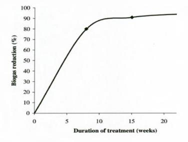
Figure 5.19: Reduction of biogas potential as a function of the duration of the forced aeration treatment involved in MBT (source: Modella and Lobo, 2010).
