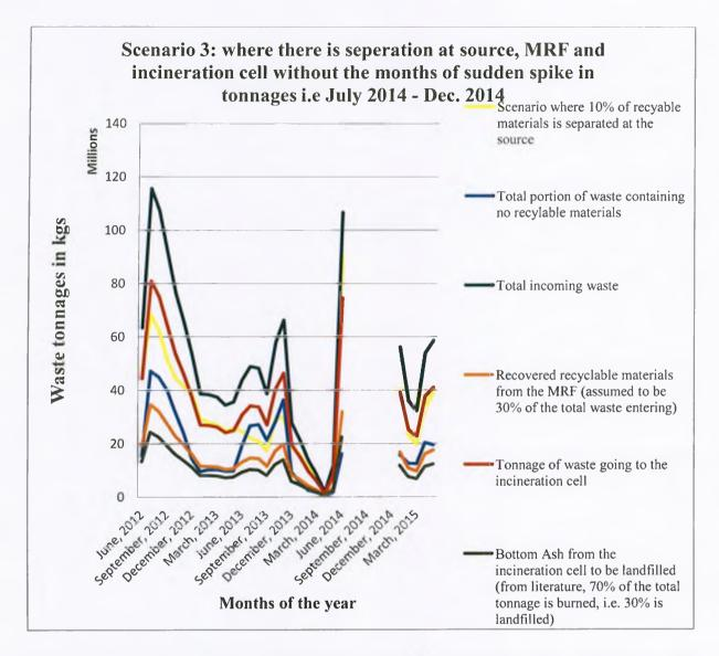
Figure 5.15: Scenario 3: 10% separation at the source, a functional MRF and an incineration cell without the months of sudden spike in tonnages i.e July 2014 - Dec. 2014
