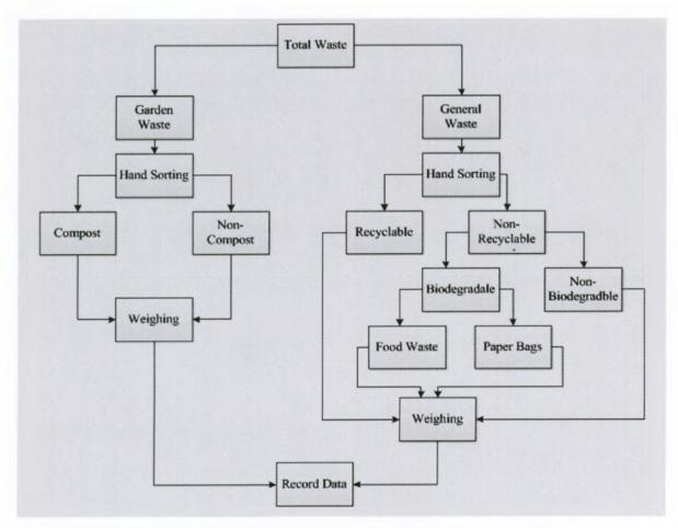
Figure 2.9: Waste Characterization Flow Diagram (Source: Sebola et al., 2014)
