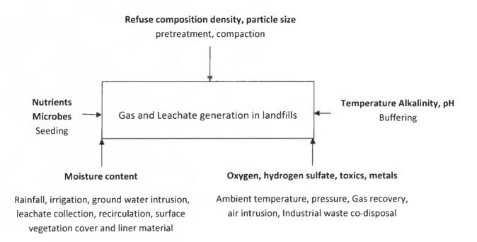
Figure 1.1: Factors influencing gas and leachate generated in landfills (After: El-Fadel et al., 1997)
