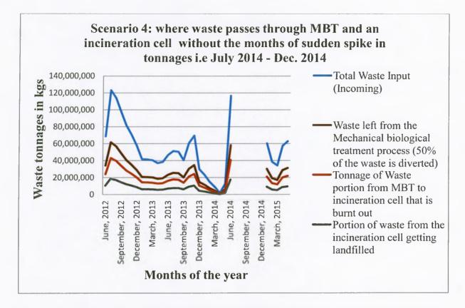
Figure 5.18: Scenario 4 – Waste passes through MBT and an incineration cell without the months of sudden spike in tonnages i.e. July 2014 – Dec 2014
