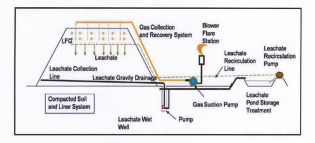
Figure 2.5: Components of a Bioreactor Landfill (Source: Mudua, 2012)
