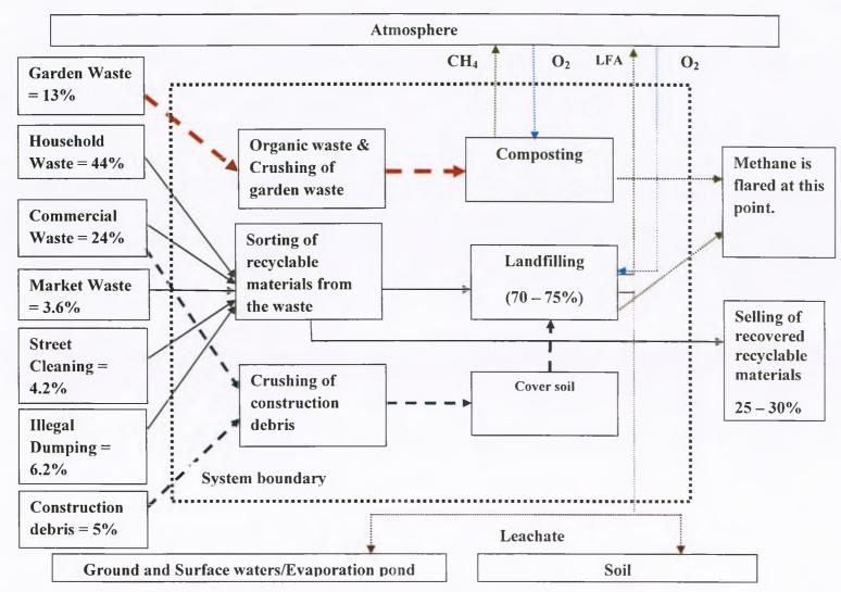
Figure 5.5: A breakdown of the material flow in Robinson Deep Landfill
