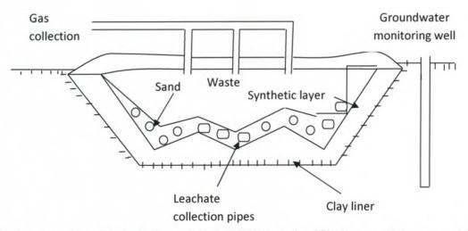
Figure 2.4: Cross section of a typical municipal solid waste landfill (Source: Masters and Ela, 2008)
