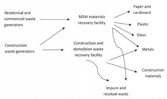
Figure 2.3: A recycling system including the waste generators, material recovery facilities, and markets for recovered material (Source: Mihelcic and Zimmerman, 2010)
