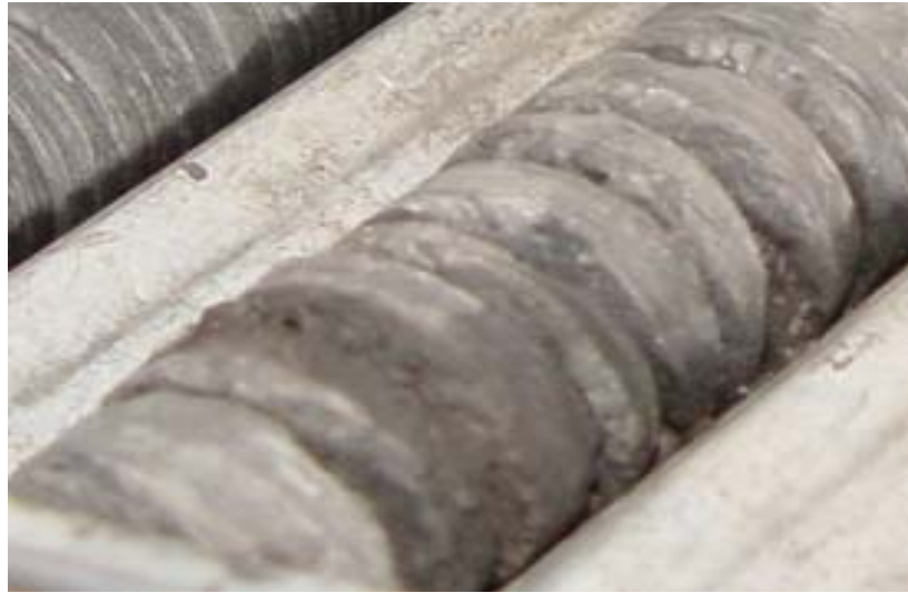
Figure 3.18: Disced core from one of the guttering sites
