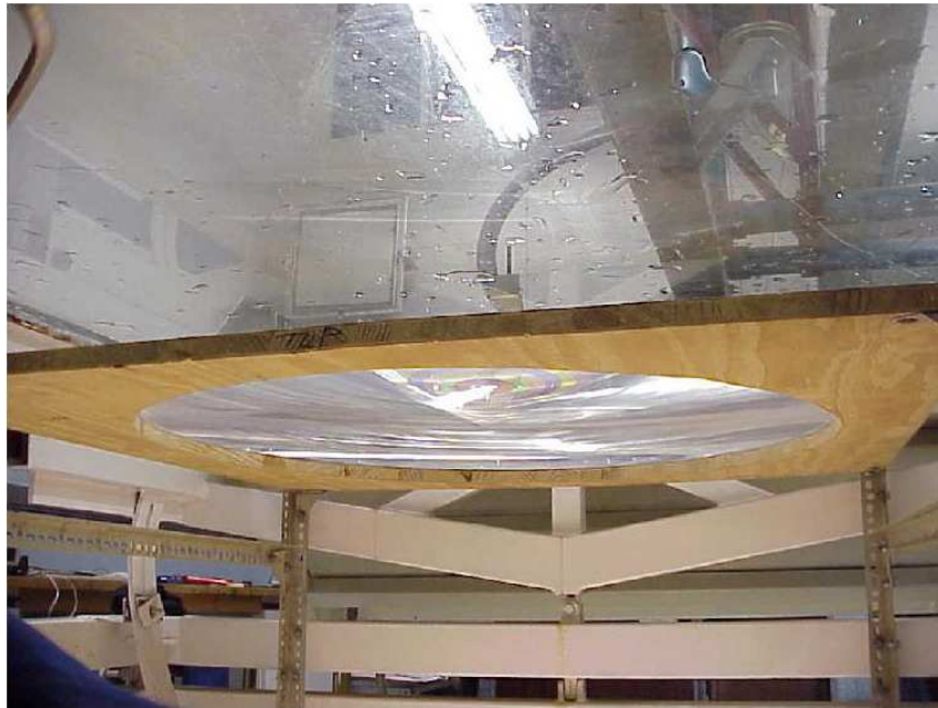
Figure 7.3: The Fresnel lens situated beneath the water table
