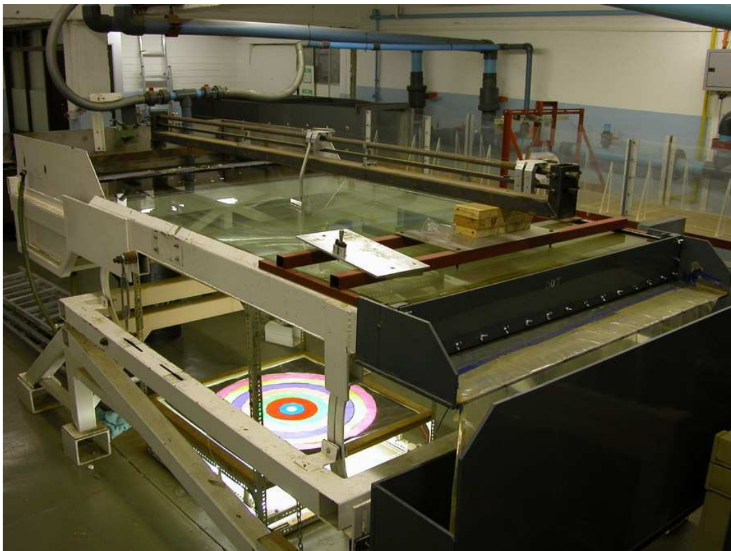
Figure 7.1: The water table facility
