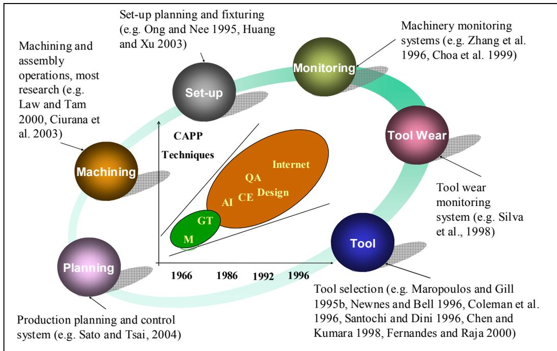
**Figure 2.2** CAPP domains and techniques evolution and diversification (“M” Machining, “GT” Group Technology, “QA” Quality Assurance, “CE” Concurrent Engineering)
