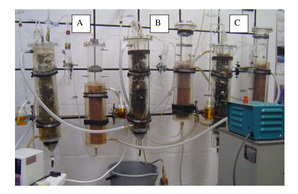
Figure 2.2.1. Reactor set-up for reactor sets A, B and C. Set A: no nutrient addition to the soil; Set B: 50  $\mu$ M nitrate and 150  $\mu$ M phosphate concentrations and Set C: dried sewage sludge cake added to soil.
