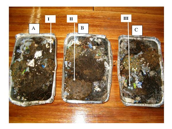
Figure 2.2.2. Wastes from anaerobic reactors A, B and C after run completion. (I) Degraded organic matter (fruit, vegetables, meat, etc.). (II) Paper content. (III) Plastic content.
