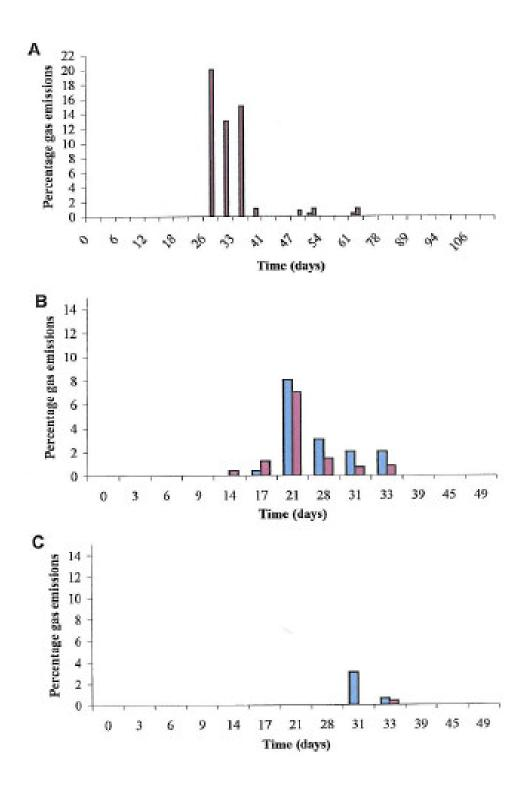
Figure 2.2.4. Gas chromatography analysis of methane  $(CH_4)$  and carbon dioxide  $(CO_2)$  of gas samples from anaerobic reactor Set A (A) and Set B (B) and Set C (C) in comparison.
