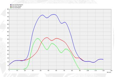
An observation of the configured client nodes indicates that none of the rejected calls originated from or was destined to the privileged users. All the observed call rejections were at the public and eyewitness client nodes. At the end of the crisis situation (800-1 200 seconds) the network reverts to its default state where no call rejections are observed and all call initiation requests are successful.
