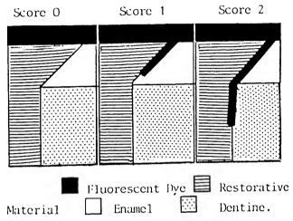
Fig. 1 Experimental Marginal leakage scoring system.
