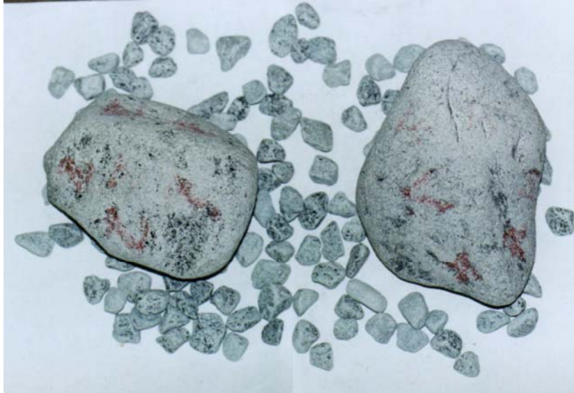
Figure 3-2 Large media rocks (-126 +106mm) that have spent over 90 min in the mill and a fine fraction (-16 +13.2mm) that has been in the mill for about 20 minutes.
