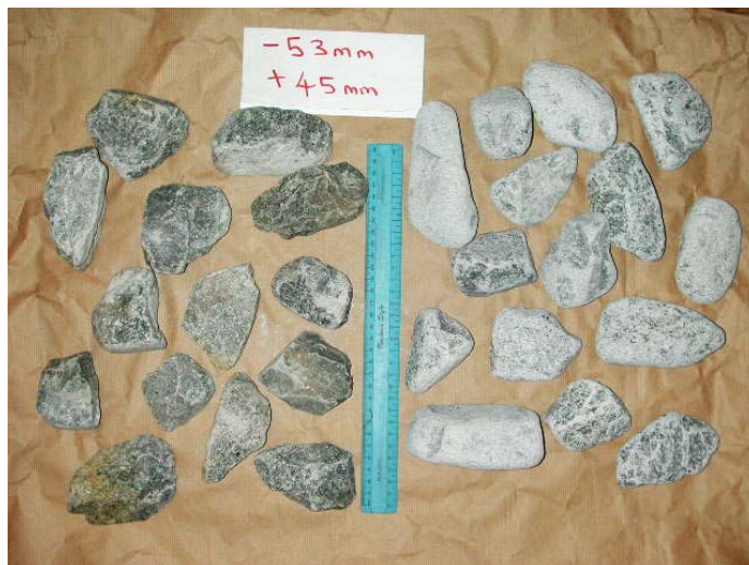
Figure 3-1 Sample of raw material on the left of the ruler and sample that has been tumbled in the mill for about 30 minutes on the right
