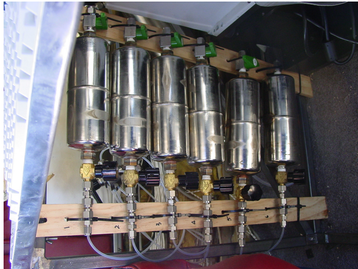
Figure 2.5 Canisters connected inside the plane for the collection of VOCs samples.
