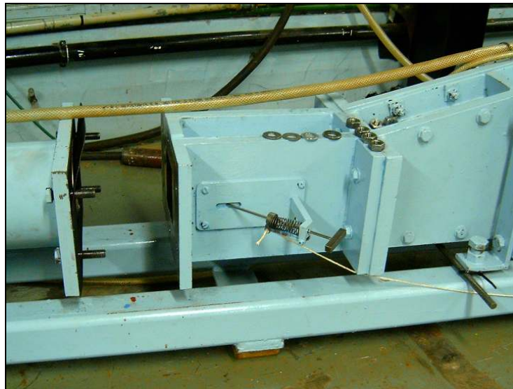
Figure 3.6 – Plunger Section showing separated driver section to the left, the armed plunger in the centre, and divergent section to the right.
