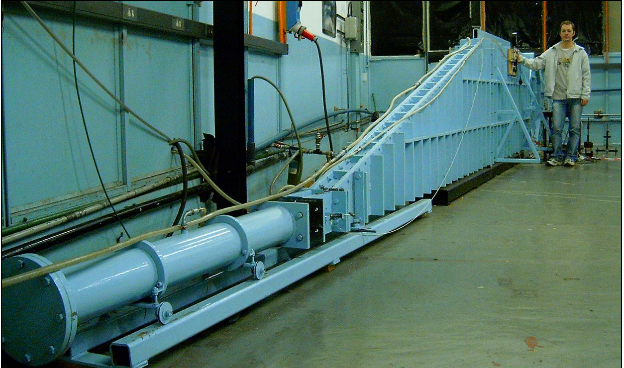
Figure 4.1.3 – Photograph of complete shock tube with the author standing next to the rig to demonstrate the scale of the equipment. The driver can be seen in the foreground.
