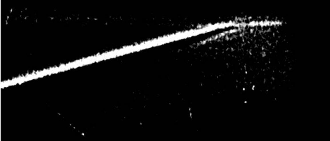
Figure 6.11 - Photograph number A16, M_{12} = 1.063 , M_{34} = 1.094 , Mach stem length = 727 mm
