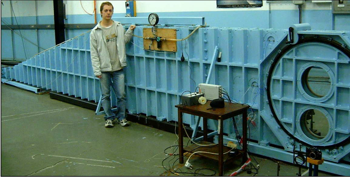
Figure 4.1.4 – Another view of the completed shock tube. The test section windows can be seen to the far right.
