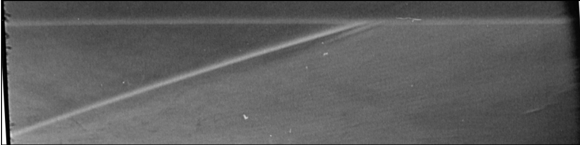
Figure 6.4 – Photograph A08, M_{12} = 1.073 , M_{34} = 1.093 , Mach stem length = 766 mm
