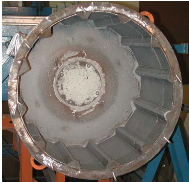
Figure 3.1 Mill lifters configuration
