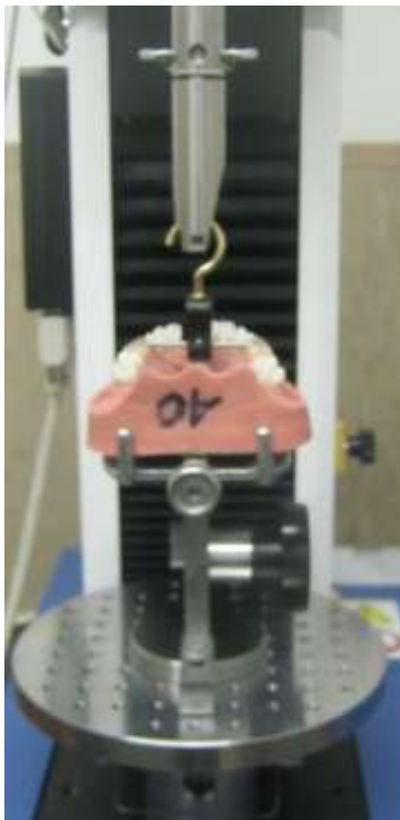
Figure 5 Typodont model on custom-made platform on universal testing machine with hook in place on upper jig.
