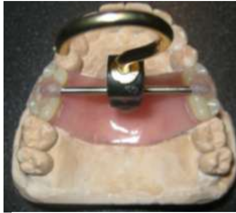
Figure 2 Acrylic partial denture with hooking device to enable placement in a universal testing machine.
