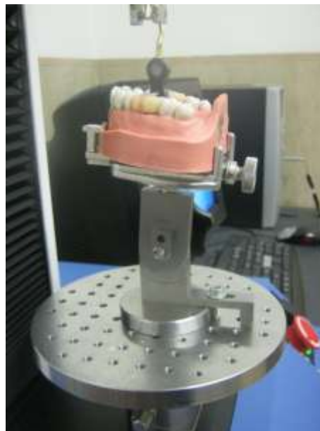
Figure 3 Side view of lower jig made to take a model platform from a model surveyor.
